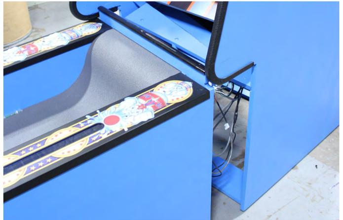
Push the ramp cabinet to about a foot from the target cabinet, and plug in the six sets of cables as shown. The phone cable linkage can be found in the cashbox of the game.
