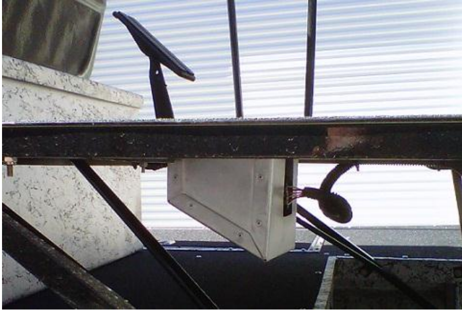
Figure 15: DBW Foot Pedal Installed
