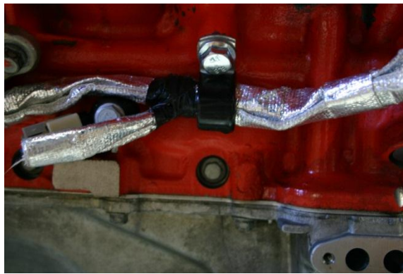
Figure 21: Driver's Side Rear P-Clip Installation
