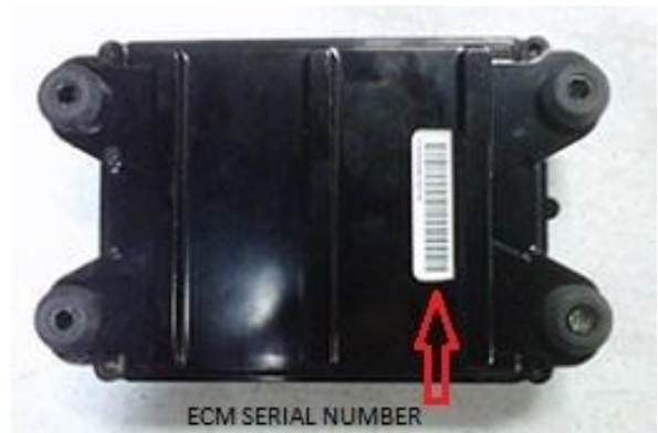
ECM Serial Number located on Back of M-90 WBO2 ECM
