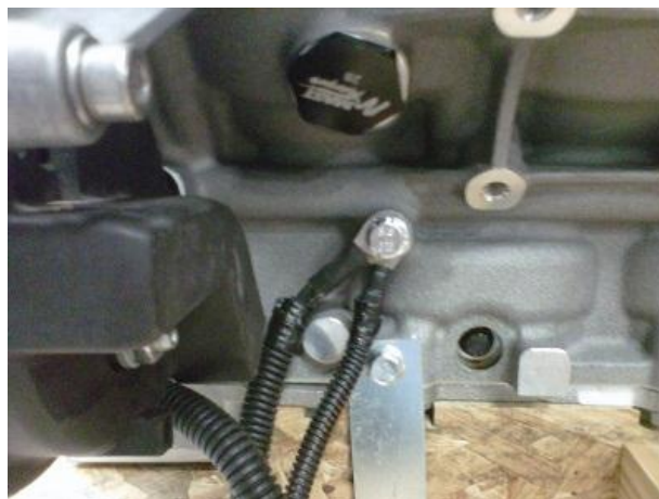
Figure 17: M-90 ECM and Fuse Block Ground Terminal Installation
