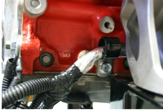
Figure 20: Driver's Side Front P-Clip Installation
