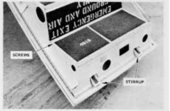
Figure 4. (above left) By placing a combination square (A) against the latch hook (B), a measurement of the hook's upward travel can be made with a feeler gauge. Figure 5. (above right) The hooks latch on the stirrups.
