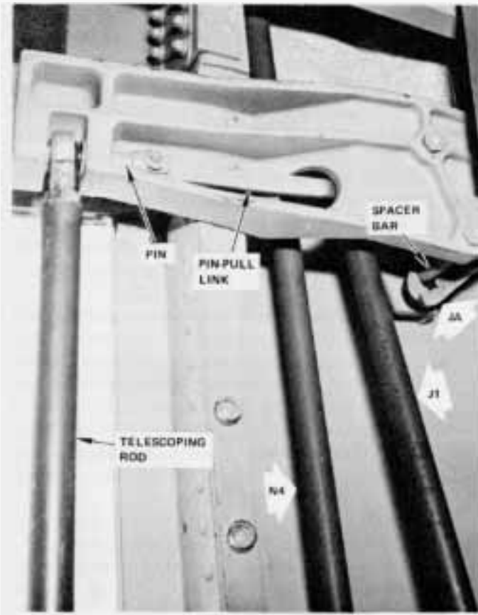
Figure 9. The function of the pin-pull assembly is to release the telescoping rod when the door is jettisoned.
