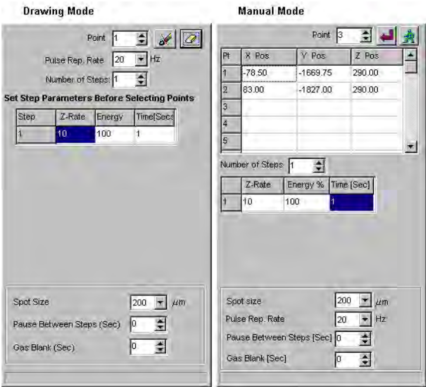
Figure 15. Depth Profile Method in Drawing mode (left) and Manual mode (right).
