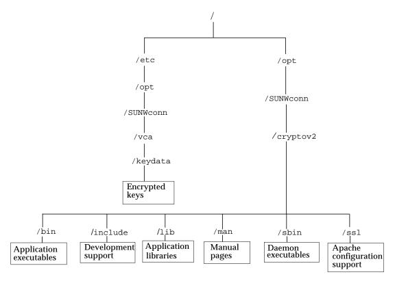
FIGURE 2-1 Sun Crypto Accelerator 4000 Directories and Files
