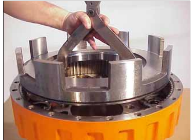
Figure 35 Set pressure ring into position. A lifting device similar to the one shown can ease installation. Refer to tool drawing on page 30.
