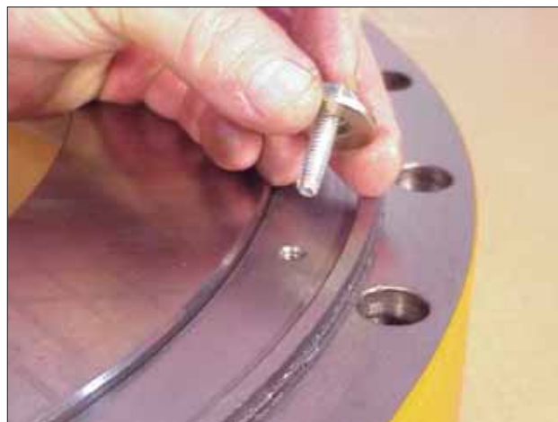
Figure 15 Place brake cover on flat surface face down. Install (3) screws and flat washers in the brake piston puller holes. CAUTION: Brake cover is heavy and can cause injury and damage.
