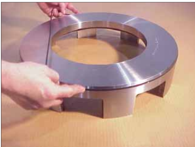
Figure 34 Lubricate seal ring with grease and install on pressure ring.
