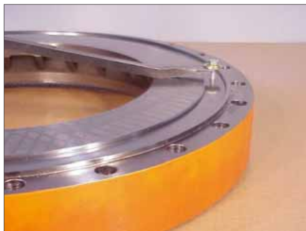
Figure 17 Using a pry bar, evenly pry piston out of the brake cover until it is no longer in contact with the piston seals.
