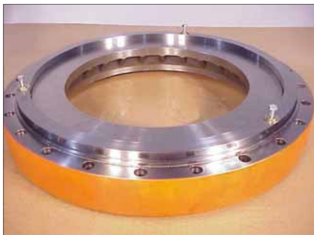
Figure 18 Piston pulled out of seals. Piston can be removed by hand at this point.
