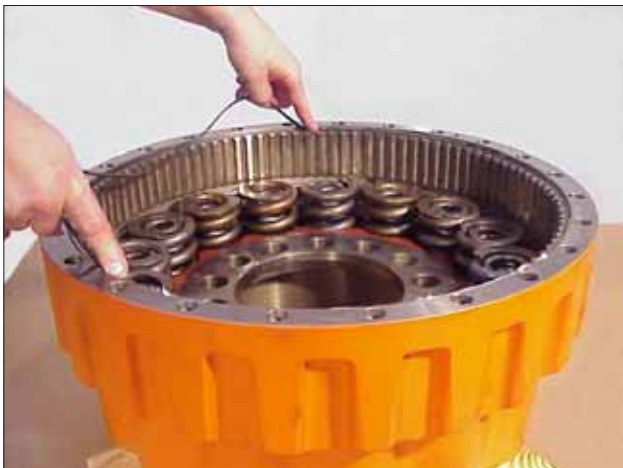
Figure 33 Lubricate brake cover seal ring with grease and install.
