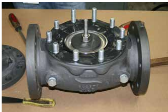
Figure 9 – Cover Spring Removal
