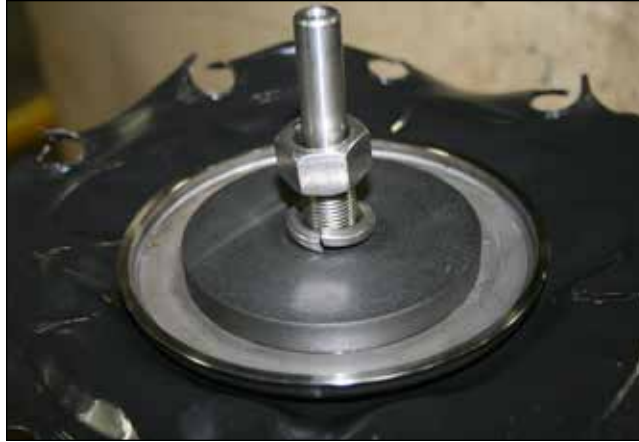
Figure 13 – Stem Nut Removal
