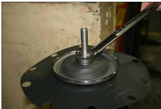
Figure 26 – Engaged Lock Washer
