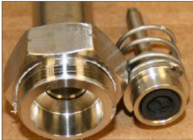
Figure 4 – Solenoid Elastomer Damage Example
