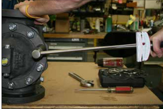
Figure 35 – Torque Cover Nuts
