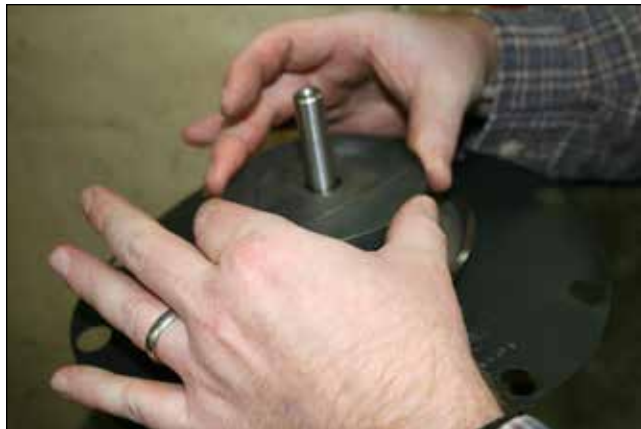
Figure 24 – Back-up Plate Installation
