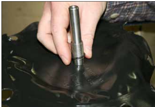
Figure 15 – Diaphragm O-ring Removal
