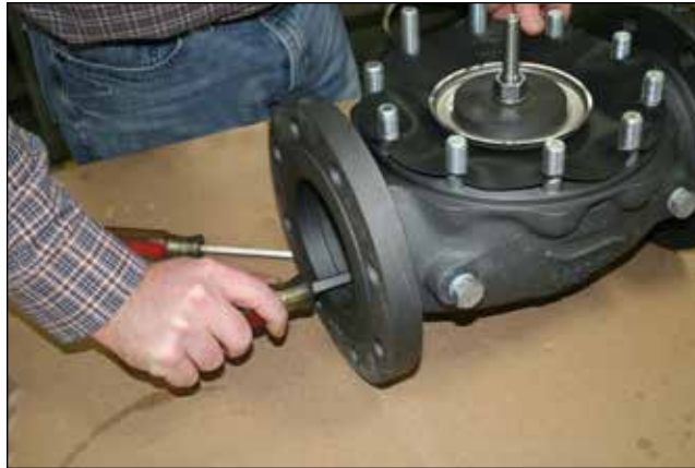
Figure 29 – Stem Assembly Installation
