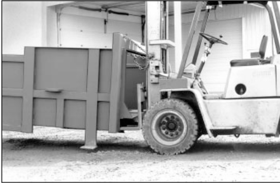
Lifting a compactor from the chamber end.
