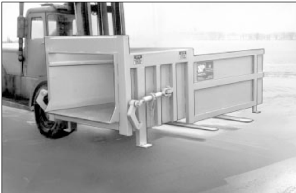
Lifting a compactor from the side.
