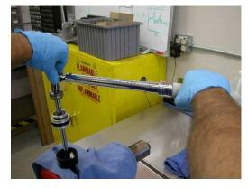
5. Clamp the impact body of the shock securely in the vice, with the open end of the body facing up.
