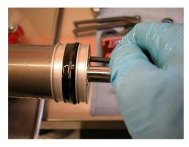
26. Using the hammer and pin punch, carefully tap a new nylon ball into the hex of the nitrogen valve pellet retainer. (Picture 22) Be extremely careful not to strike the surface of the shock body and damage it with the hammer.
