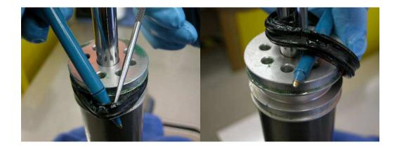
17. Using the point of the scribe, remove the nylon ball from the nitrogen filler valve on the shock body. (Picture 6)
