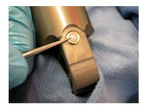
18. Insert the FOX Nitrogen Safety Needle into the nitrogen filler valve on the shock body and, using a small blunt object such as and allen wrench to depress the Schrader valve, release <u>all</u> of the nitrogen pressure. (Picture 7)
