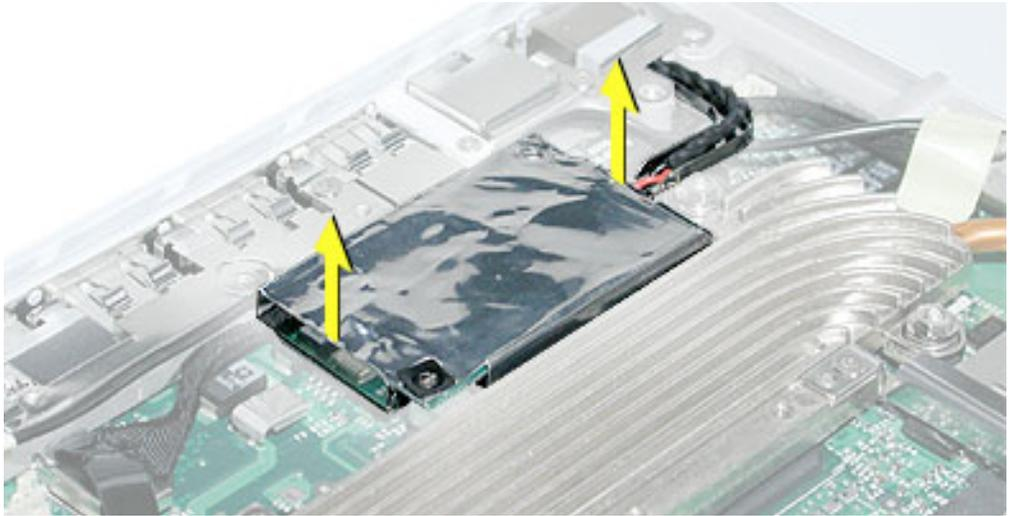
4. Disconnect the cable from the upper end of the modem board.
