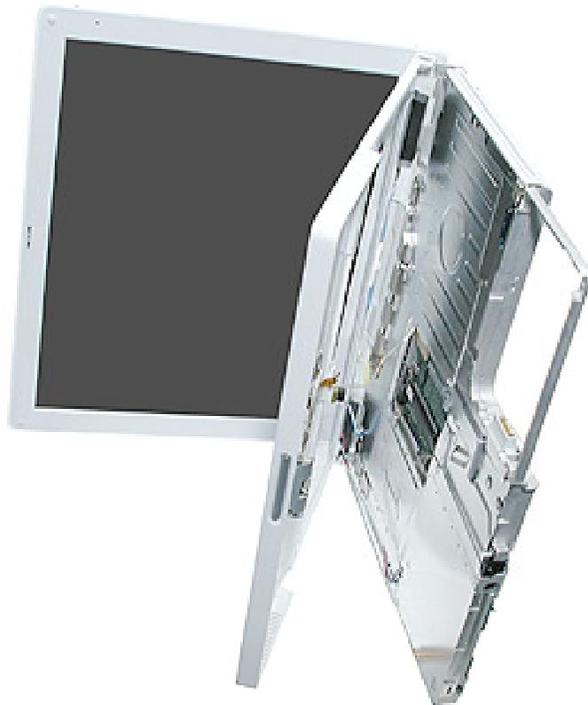
12. Place the computer upright, and move the top case off center. Use a black stick to carefully disconnect the two cables from the logic board.
