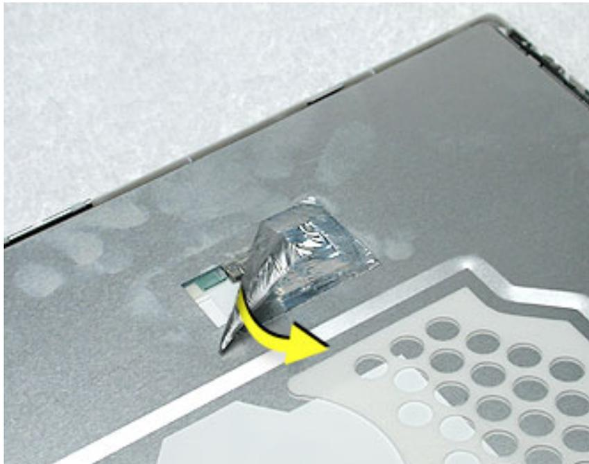
8. Peel up the tape if it covers the two screws at the clutch. Remove the two Phillips screws.
