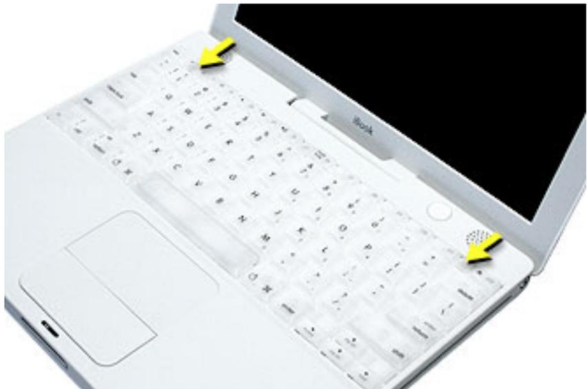
4. Flip the keyboard over and lay it on the palm rest.
