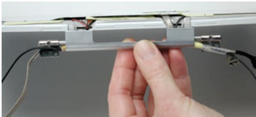
**Note:** The clutch caps are mirror images of each other. There is a right clutch cap and a left clutch cap. Note the positioning of the clutch caps on the display clutch cover. The image below shows the left clutch cap installed.
