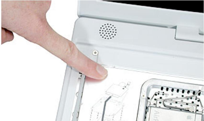
2. Lift up the flexible wire bracket that secures the card.
