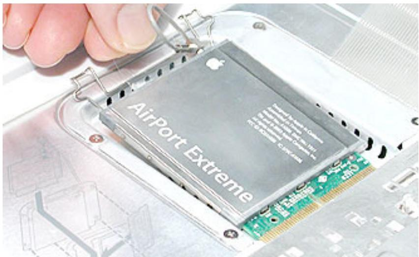
7. If an AirPort Extreme Card is not installed, unlatch the flexible wire bracket to release the AirPort antenna cable.
