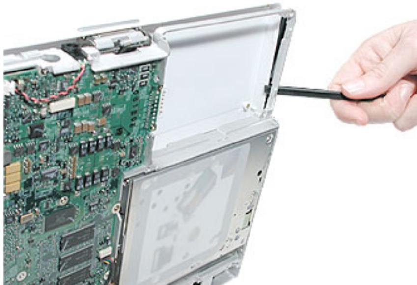
9. As you begin to loosen the top case, check that the trackpad cable (orange flex cable) has disconnected from the top case. Or use a black stick to disconnect it.
