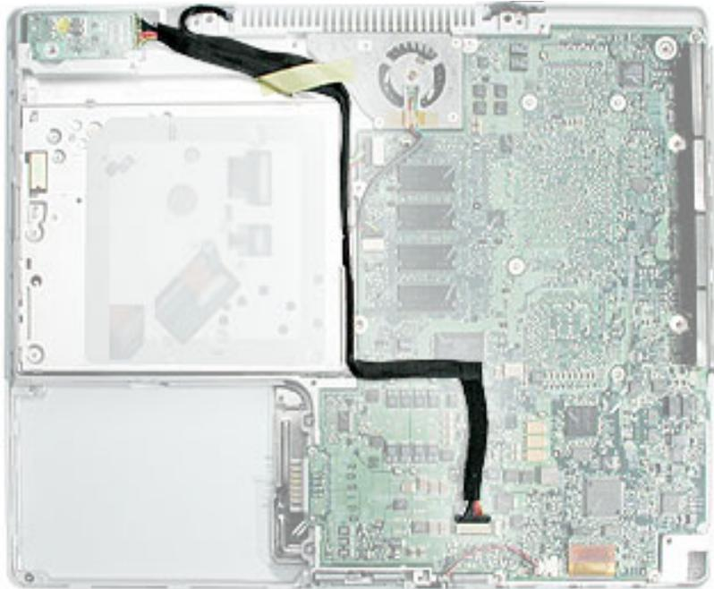
4. Remove the two identical screws from the DC-in board.
