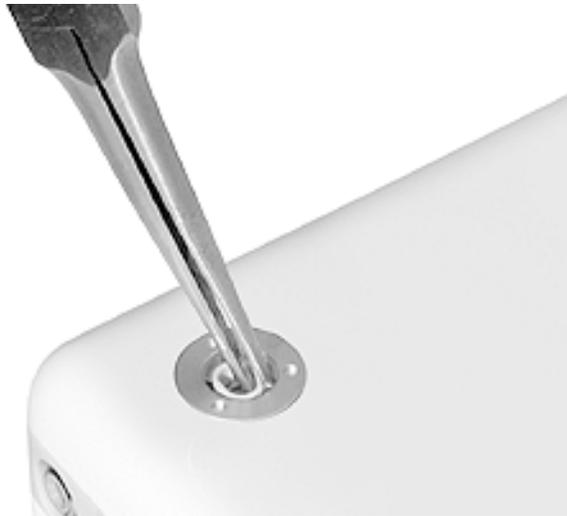
6. Use a screwdriver to remove the screw and socket from the bottom case.
