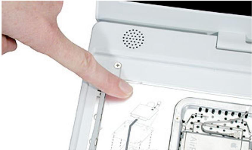
6. If the computer has the optional AirPort Extreme Card installed, unlatch the flexible wire bracket that secures the card.
