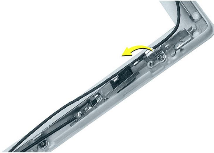
7. At the bottom of the bezel, remove the tape from the inverter board and note the routing of the two soldered cables on the left side of the antenna board.
