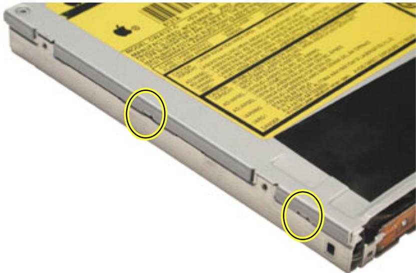
6. Replace the four screws. If applicable, install the brackets, cable, and faceplate back on the drive before returning the old drive.
