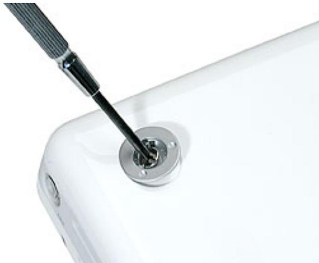
7. Install the new socket. For the best fit, do not reuse the old socket.
