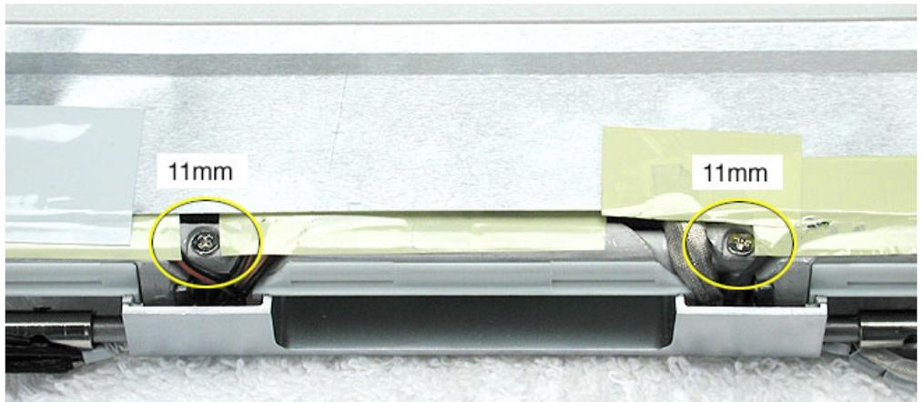
9. Peel up the tape that anchors the folded mesh strip of the LCD cable to the shield.
