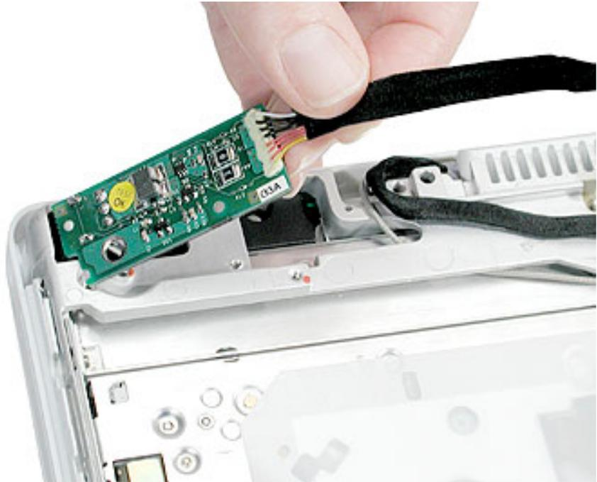
6. Remove the DC-in board from the computer assembly.
