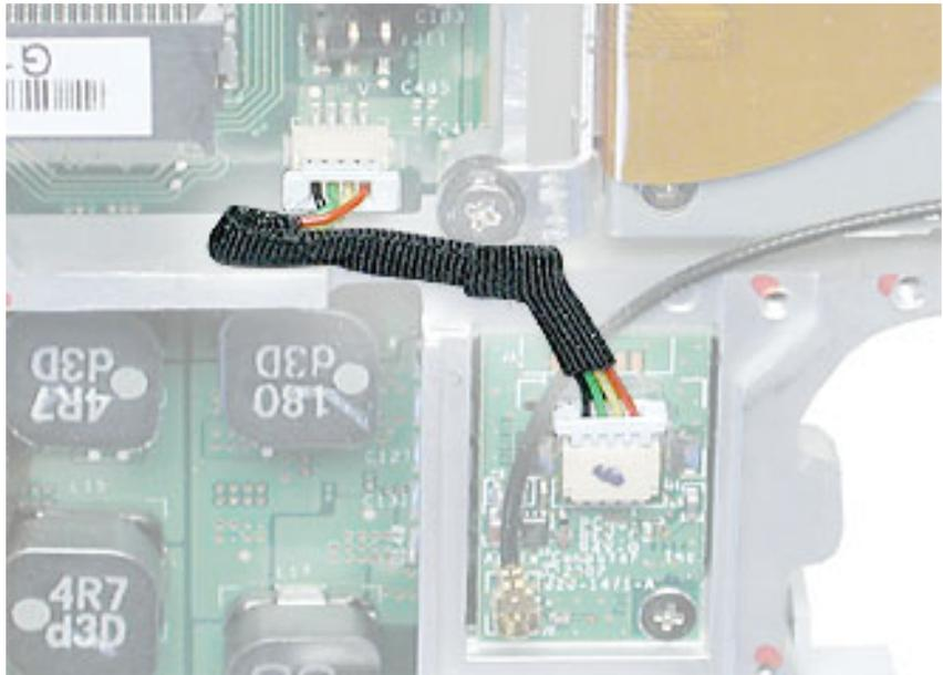
2. Disconnect the antenna cable from the Bluetooth board.
