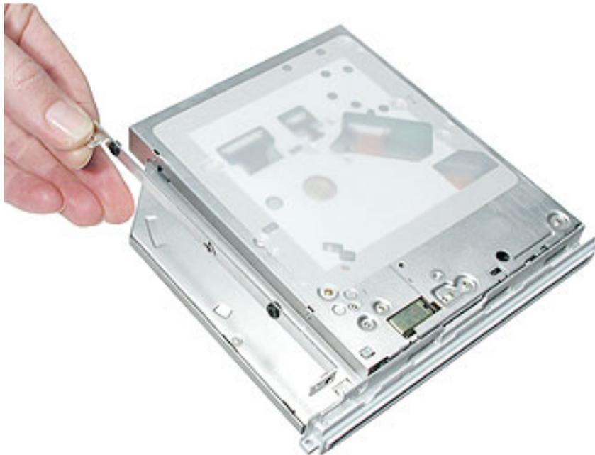
11. **Caution:** The bezel and optical drive case is a soft material. Be especially careful when removing the bezel from the optical drive.
