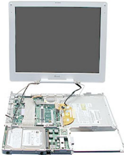
10. Install the replacement display module, and reassemble and test the computer.
