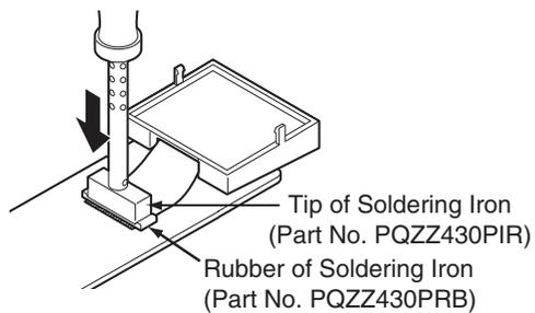
Heatweld with the tip of the soldering iron about 5 to 8 seconds (in case of 60W soldering iron).
