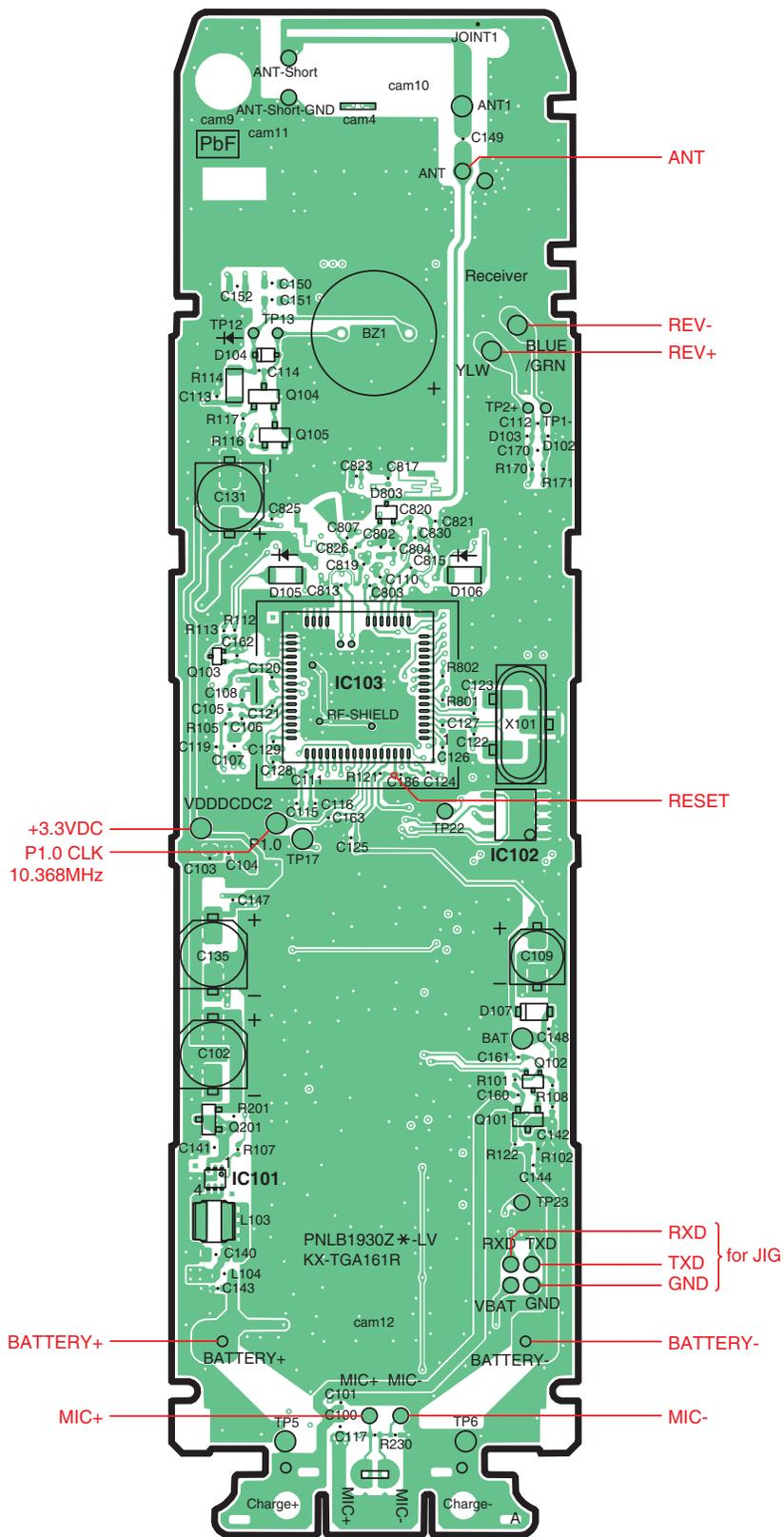
KX-TGA171 CIRCUIT BOARD (Handset\_Main (Component View))
