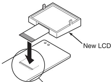
Fit the heatseal of a new LCD.
