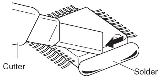
3. While the solder melts, remove it together with the IC pins.
