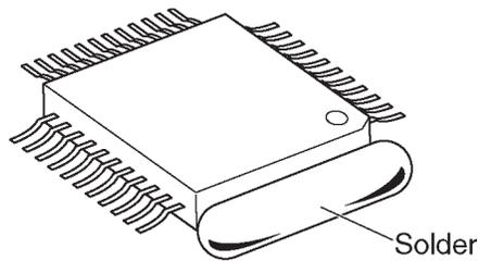
2. Make a few cuts into the joint (between the IC and its pins) first and then cut off the pins thoroughly.
