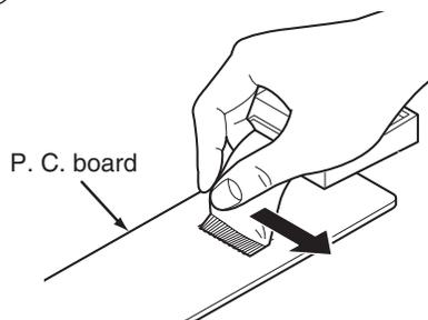
Peel off the FFC (Flexible Flat Cable) from the LCD, in the direction of the arrow. Take care to ensure that the foil on the P.C. board is not damaged.
