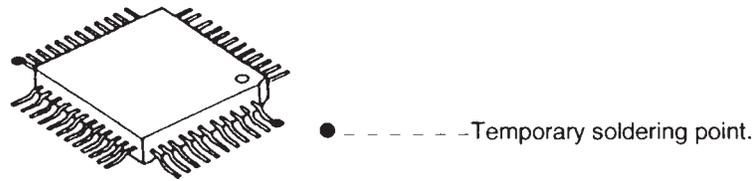
\*Check the accuracy of the IC setting with the corresponding soldering foil.
