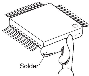
When you attach a new IC to the board, remove all solder left on the board with some tools like a soldering wire. If some solder is left at the joint on the board, the new IC will not be attached properly.
