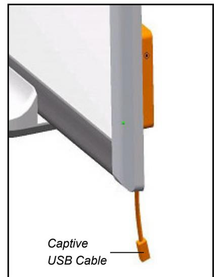
**To connect using a USB cable**
