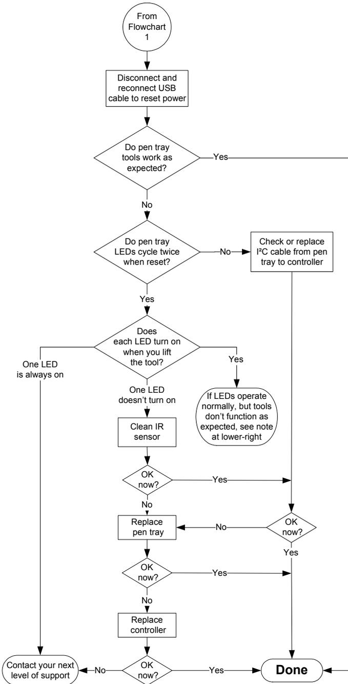
When you disconnect and reconnect the USB cable to reset the power as described in *Resetting Your Interactive Whiteboard* on page 41, all of the pen tray LEDs flash sequentially twice, indicating successful communication with the controller. If they flash continuously, contact your next level of support.
