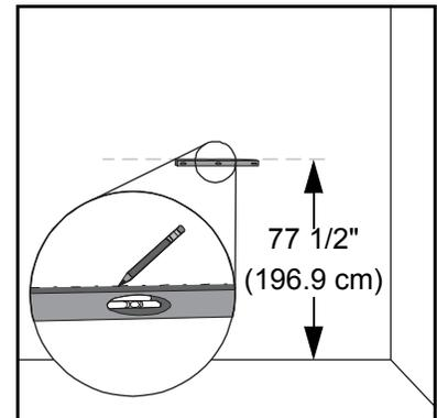
2. Using the mounting bracket as a template, mark the location of the five mounting holes on the wall.
