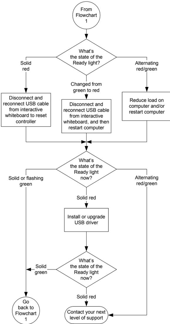
Disconnect and then reconnect the USB cable at both ends to reset your interactive whiteboard and re-establish the connection.
