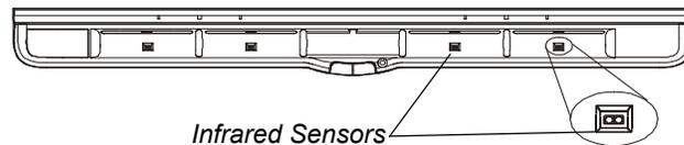
To clean a sensor, moisten a cotton swab with a household glass cleaner, such as Windex, and then carefully clean the infrared transmitter and receiver.
