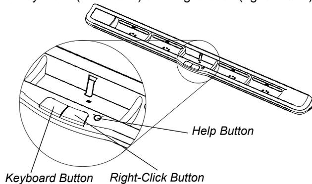
You can customize the buttons using SMART Product Drivers to provide several other functions, including printing, changing pages and capturing the screen. Pressing both buttons simultaneously starts the orientation process.
