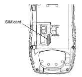
If your SIM card is not in the SIM card holder, it may be in the box your phone came in, attached to a piece of plastic about the size of a credit card. If this is the case, carefully detach your SIM card from the surrounding plastic and insert it as described in "Inserting Your SIM Card" on page 14.
