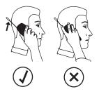
Important: Failure to fully extend or retract the antenna until the antenna clicks into place causes severely degraded performance, which may result in missed calls, dropped calls, or garbled audio.
