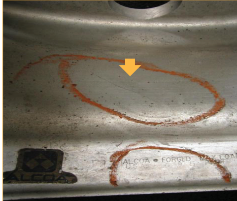
Drop center crack
