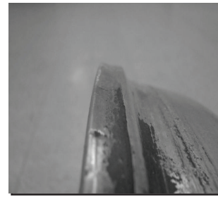
Photo 9. Sharp edge removed.
