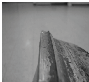
Photo 8. Severe rim flange wear.
