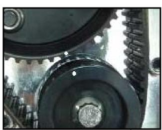
Note: Wood Performance has special tools for removing and installing the cam gear and crank gear assemblies. Use WT-001 for installing the cam gear and WT-002 for removing the cam gear. Use the WT-003 tool for removing the crank gear. When using the WT-001 tool, you need only to tighten the cam gear onto the camshaft until it is fully seated. Do not torque at this time. (See Picture #5)
