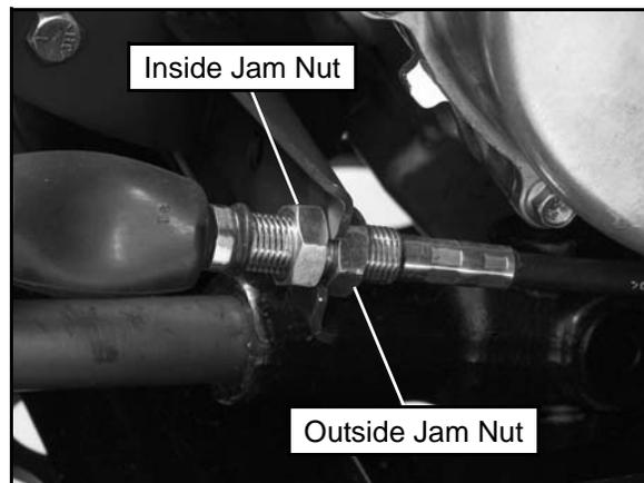
4. After turning the outside jam nut 1 1/2 turns. Hold the outside jam nut with a wrench and tighten the inside jam nut clockwise, until it is tight against the bracket.
