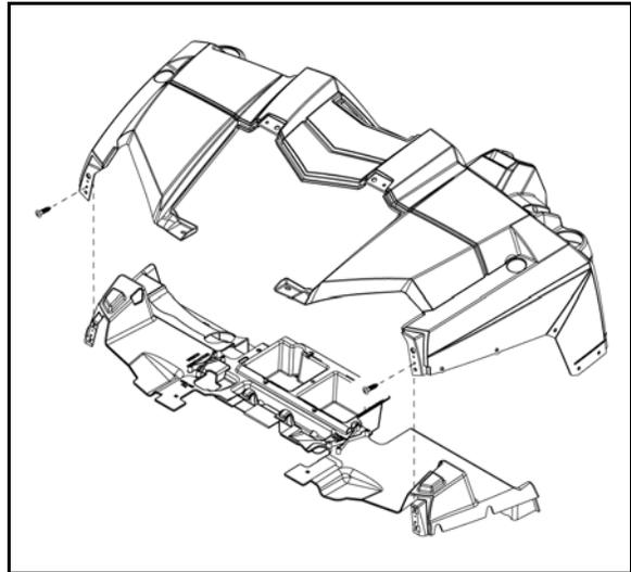
5. Remove the (11) remaining screws and (6) push rivets retaining the front cab.
