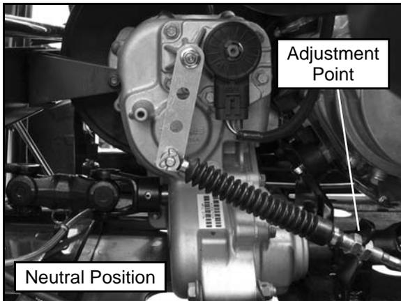
2. Locate the shift cable adjustment point attached to the frame in front of the transmission.
