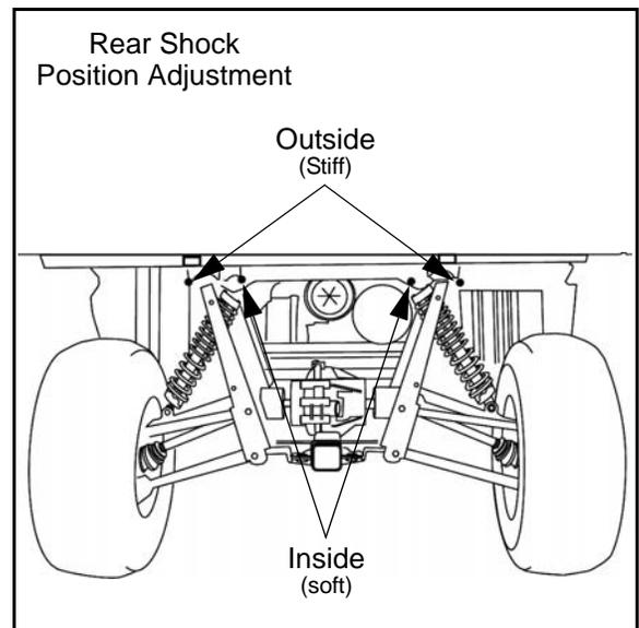
4. Reinstall the shock mounting bolts and torque to specification.
