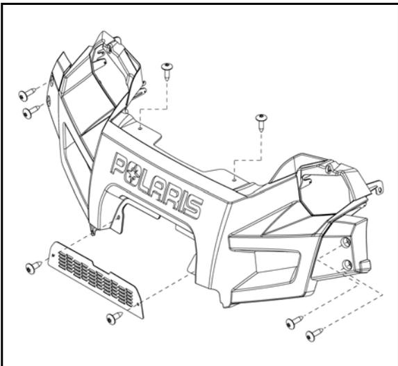
4. Remove the (2) screws that retain the front cab assembly to the hood liner.
