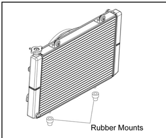
24. After the radiator is installed, be sure the mounts have remained in place.
