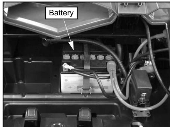
2. Remove hold-down strap and vent tube from battery.
