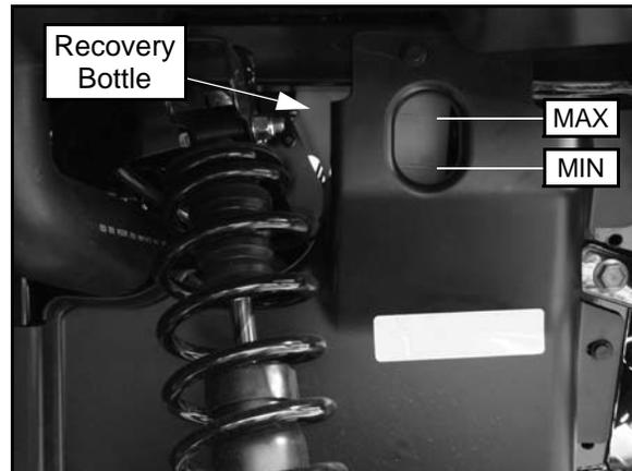
3. If the coolant level is below the "MIN" mark, open the hood to access the radiator pressure cap and recovery bottle cap.
