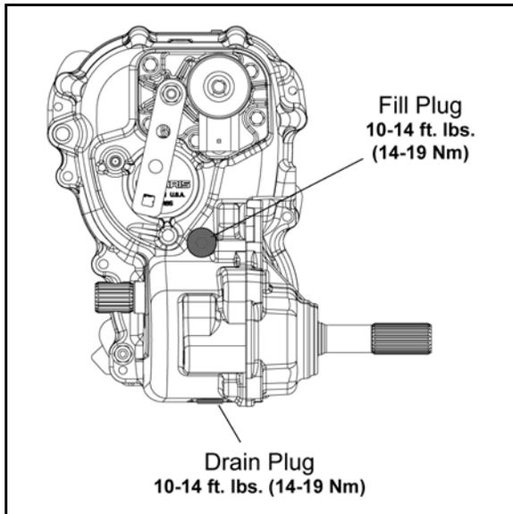
4. Clean the drain plug magnetic surface. Reinstall drain plug with a new O-ring and torque to specification.
