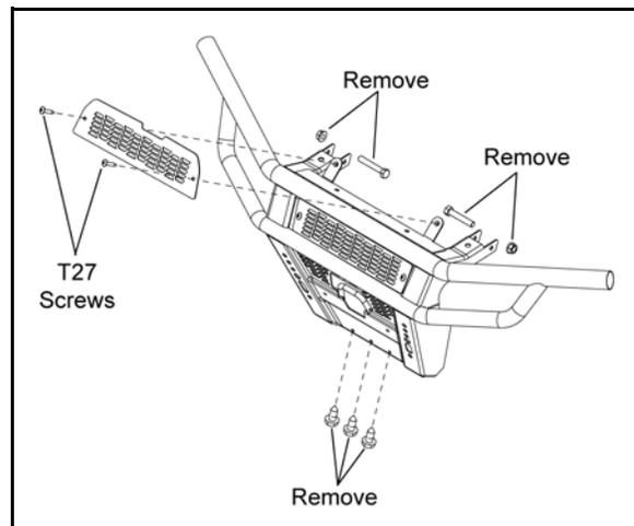
4. Remove the (3) bolts from the lower portion of the bumper.
