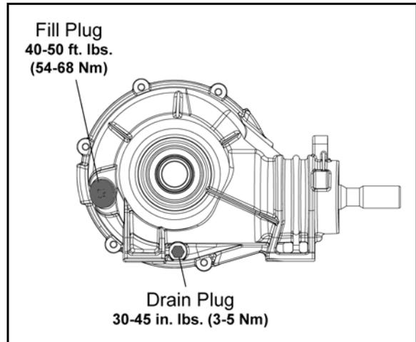
4. Clean the drain plug magnetic surface.
