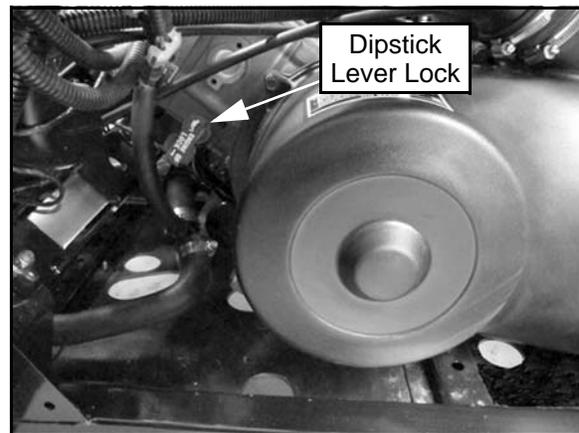
5. Reinstall dipstick and push it into place. Do not lock the dipstick.
