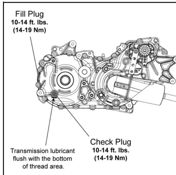
3. If lubricant level is not even with the bottom threads, remove the fill plug and add the recommended lubricant as needed. Do not overfill.
