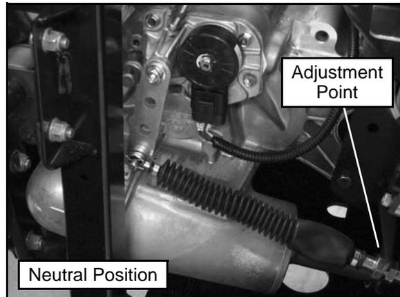
2. Locate the shift cable adjustment point at the engine-to-transmission mount bracket.
