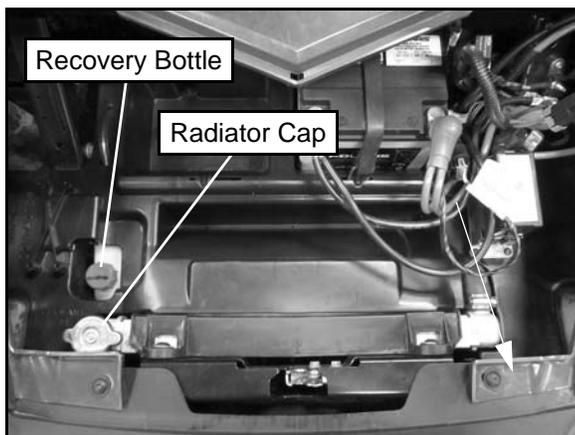
With the engine at operating temperature, the coolant level should be between the "MAX" and "MIN" marks on the recovery bottle. If not, perform the following:
