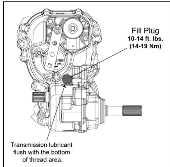
3. If lubricant level is not even with the bottom threads, add the recommended lubricant as needed. Do not overfill.
