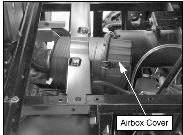
2. Unhook the (4) clips from airbox cover and remove cover. Inspect the cover seal. It should adhere tightly to the cover.
