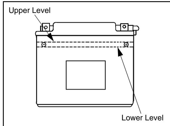
Add only distilled water. Tap water contains minerals that are harmful to a battery.
