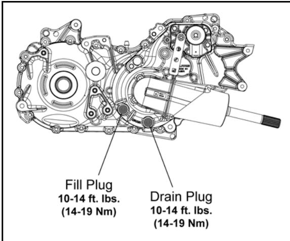
4. Clean the drain plug magnetic surface. Reinstall drain plug with a new O-ring and torque to specification.
