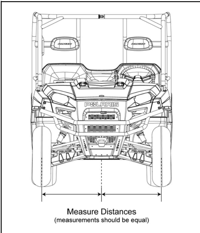
**NOTE: Be sure steering wheel is straight ahead before determining which tie rod needs adjustment.**
