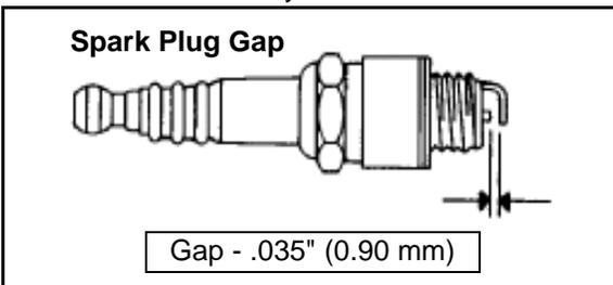
6. If necessary, replace spark plug with proper type. **CAUTION:** Severe engine damage may occur if the incorrect spark plug is used.
