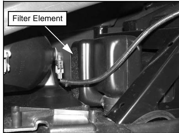
3. If the filter element is dirty, clean it with a high flash point solvent, followed by hot soapy water. Rinse and dry the filter element thoroughly. Inspect element for tears or damage. Replace if necessary.
