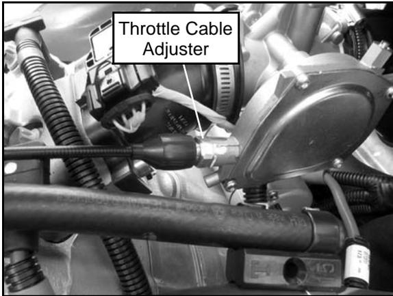
3. Slide back the cable adjuster boot.
