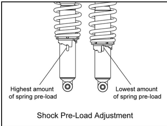
Vehicle loads effect suspension spring pre-load requirements. Use Spanner Wrench (PN 2871095) to adjust pre-load as necessary to avoid bottoming of the shocks.
