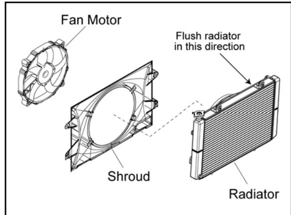
2. Carefully straighten any bent radiator fins.
