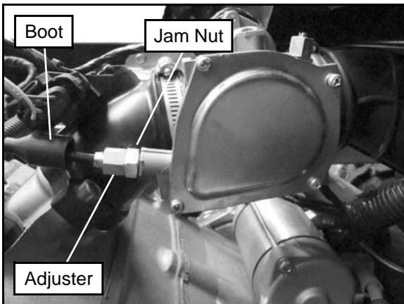
**NOTE:** While adjusting, lightly move the throttle pedal in and out.
