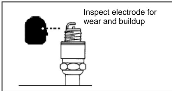
4. Clean with electrical contact cleaner or a glass bead spark plug cleaner only. **CAUTION:** A wire brush or coated abrasive should not be used.
