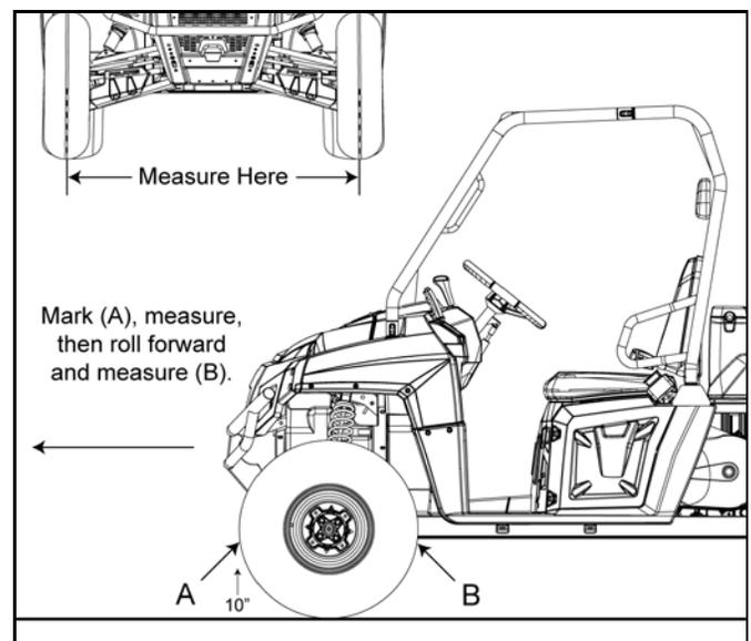
**NOTE: It is important the height of both marks be equally positioned to get an accurate measurement.**
