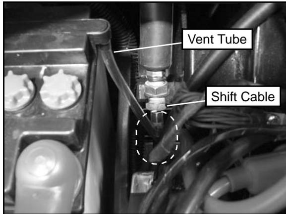
4. Route the vent tube through the triangular hole in the frame support from the back side and place it behind the panel.
