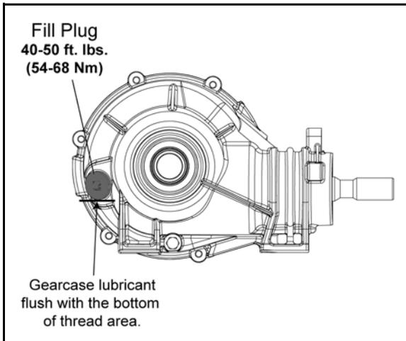
3. If lubricant level is not even with the bottom threads, add the recommended lubricant as needed. Do not overfill.
