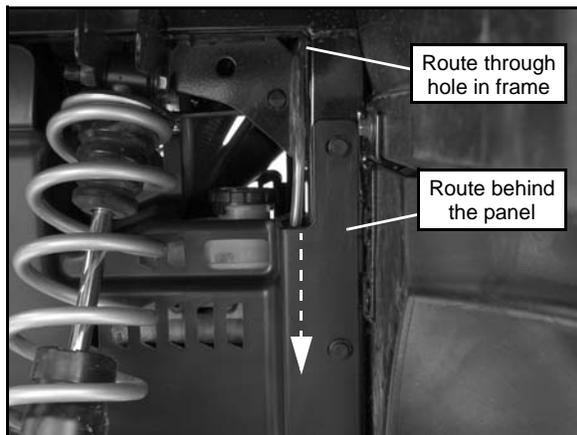
**IMPORTANT:** Route vent tube as shown to prevent electrolyte from damaging critical components (i.e. wire harness, brake lines, throttle cable).
