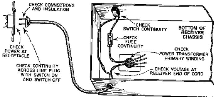
Diagram illustrating the checks which can be made for trouble in the primary a-c circuit of a receiver.
