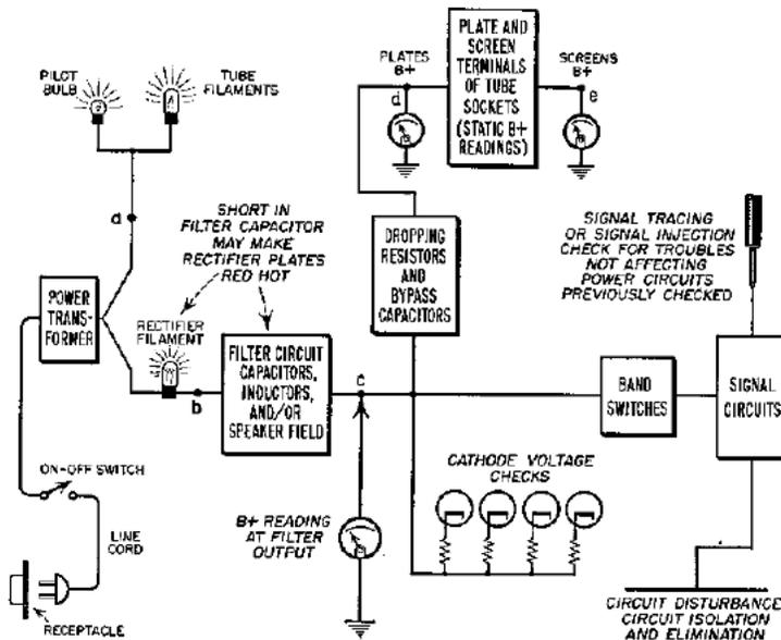
FIG. 0-2 Diagram illustrating the logical checking procedure in a dead receiver. The sequence of steps starts with the power receptacle at the lower left and proceeds toward the right as explained in the text.
