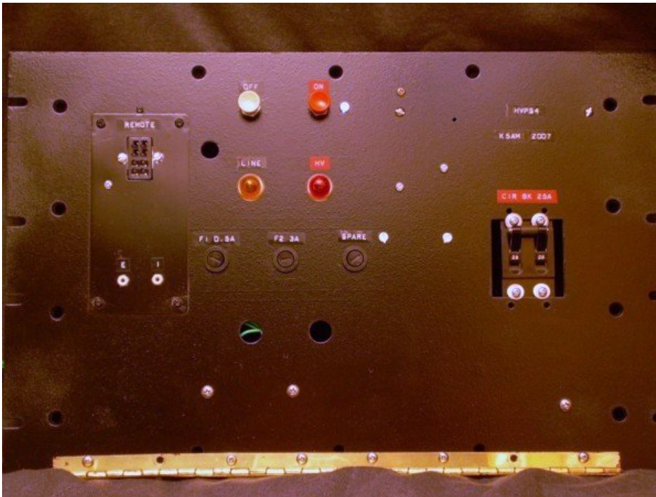
HVPS4 panel. The Jones socket is for the remote head. The push buttons and neon lamps are for local control and testing.
