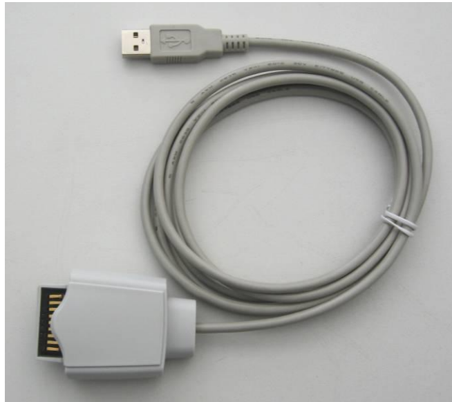
Figure 5: Screen-Connector top view
