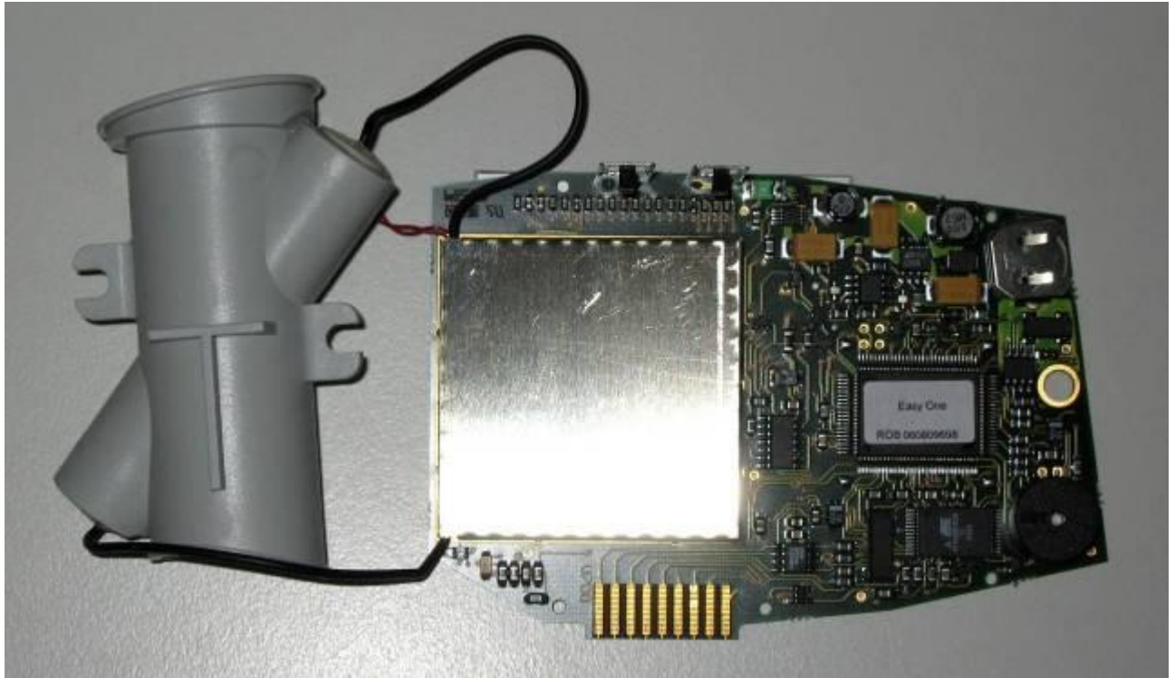
Figure 8: Top view of EasyOne-CS PCB (without EMI shielding)
