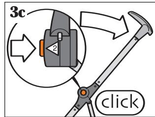
Extend the handle crossbar into the horizontal position until you hear a "click" (**Figure 3d**).
