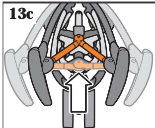
Hold onto the stroller by the hinge points and push release pedal down, and push coupling (labeled 3) forward (**Figure 13d**).
