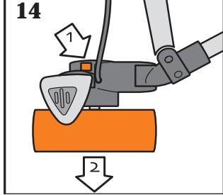
Press the release button on the bottom of each front wheel and pull wheel off of the frame (**Figure 14a**).
