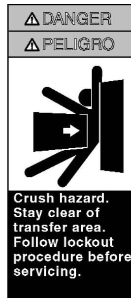
113242F0409 Crush Hazard Width 4 1/2 inch Height 9 5/8 inch
