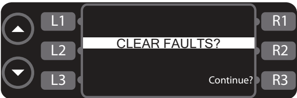
Figure 28: Confirm Clear Fault Counts Screen
