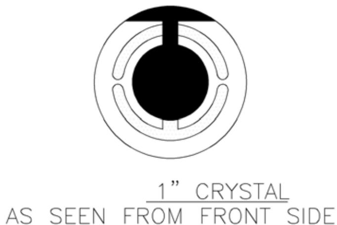
Figure 11 INFICON 1" Crystal - as Seen From The Front Side
