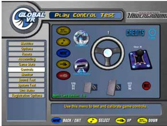
**Note:** A red dot on the lower left corner of the Attract screen indicates a hardware malfunction. Use the Play Control Test screen to determine which hardware component is not working.
