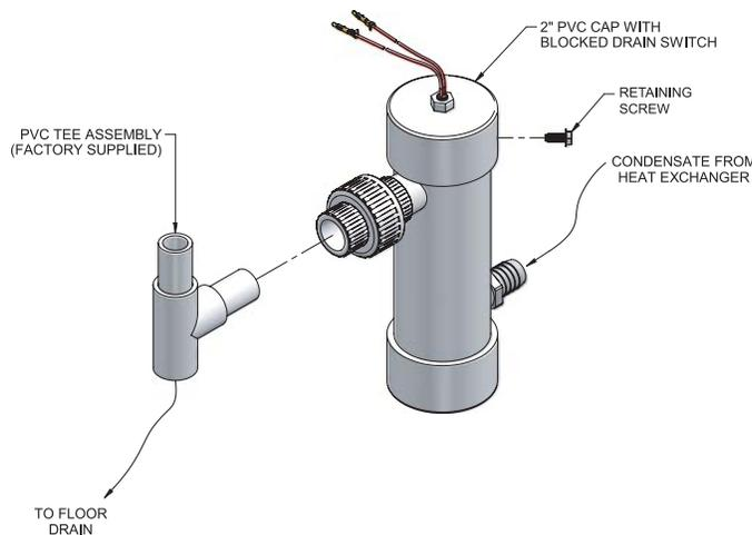
8. A condensate removal pump is required if the boiler is below the drain. When installing a condensate pump, select one approved for use with condensing boilers and furnaces. The pump should have an overflow switch to prevent property damage from condensate spillage. Call your qualified service technician to inspect the boiler and system.
