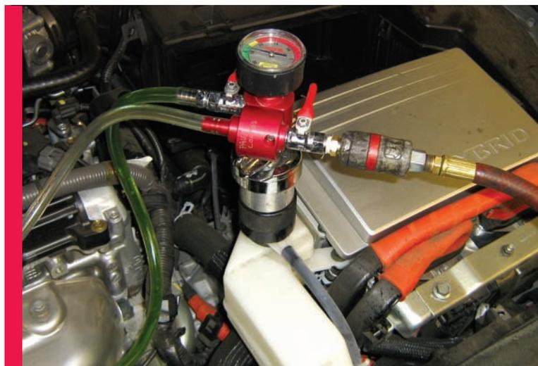
**A cooling system vacuum fill tool also works great for the inverter cooling system.**
