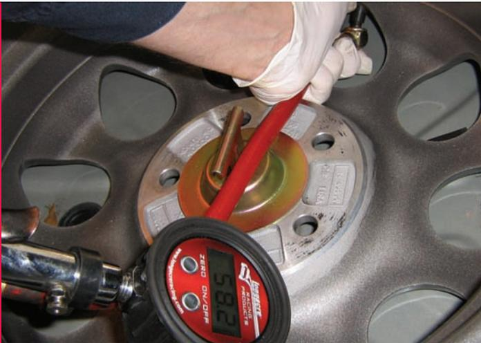
**Check and fill the Altima Hybrid spare tire pressure to 60 psi.**
