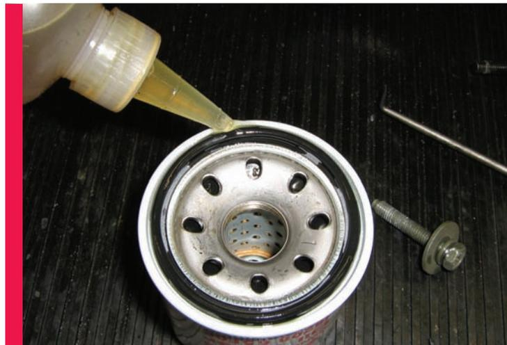
**Always lubricate the oil filter gasket with clean motor oil so it won't become stuck in place. The "next guy" may be you!**
