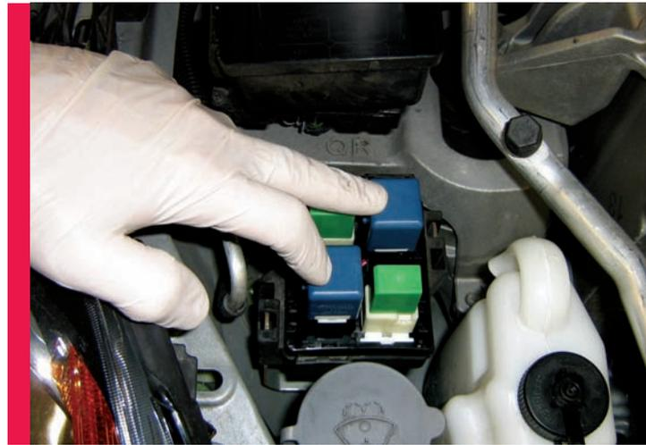
**These are the ABS Pump Motor Relays.**
