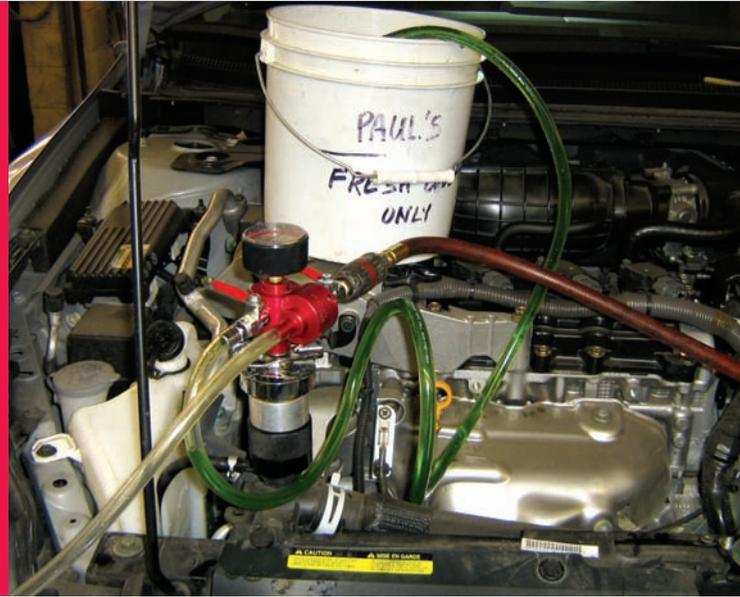
**Using a coolant system vacuum filling tool helps to eliminate potentially harmful pockets of trapped air.**
