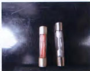
the holders. As well as being shorter, these are slightly thinner, so the contact between the holders and the fuses is quite poor. This leads to overheating of the fuse holders – clearly very undesirable.
