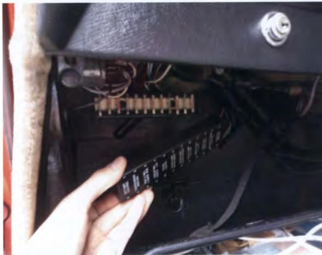
There seem to be four basic problems with the arrangement. The first is the one that generates consequences should the other three be present as well! The fuse box is made from an early nylon like soft plastic. This plastic has an extremely low melting point and also spontaneously ignites at an alarmingly low temperature. If you fancy a practical test, it should be easily possible to cause catastrophic melting with a domestic hair dryer – you might even generate a flame by this means.
