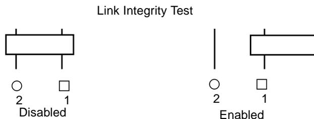
Figure 10-11 Disabling and Enabling the Link Integrity Test
