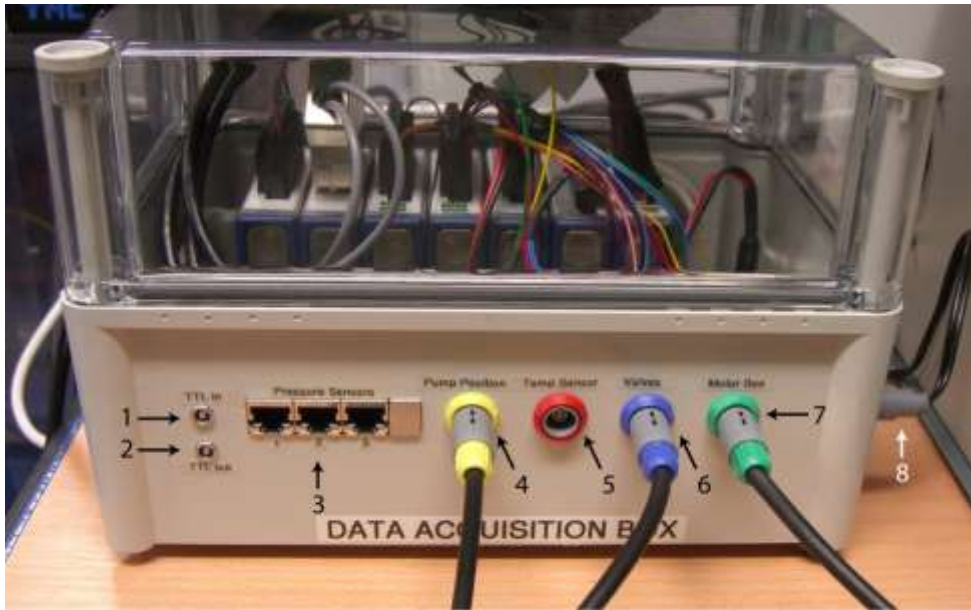
Figure 15. Photograph of data acquisition and control box. (1) TTL trigger in; (2) TTL trigger out; (3) pressure transducer sockets; (4) pressure generator linear transducer socket; (5) temperature sensor socket; (6) high pressure valve control socket; (7) motor control box interface socket, (8) power connection.
