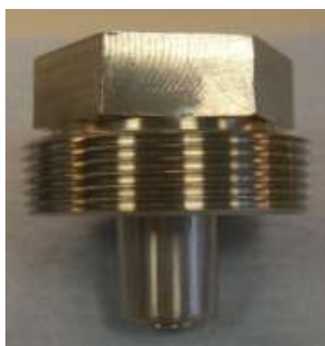
Figure 24. (Left) Photograph of O-ring sample closure. (Right) Drawing with part cross section of the O-ring sample closure.
