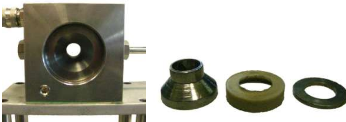
Figure 36. (Left) The pressure cell after removal of the window nuts and window support / seal assemblies. (Right) Dismantled window support / seal assembly with from left to right: window support, window packing seal and window seal washer.
