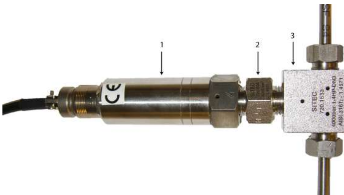
Figure 13. Photograph of pressure transducer. (1) Pressure transducer; (2) transducer coupling; (3) 3-way connector to pressure network
