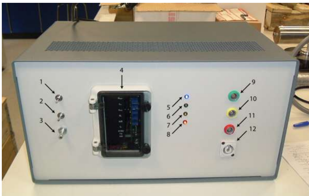
Figure 14. Photograph of motor control box. (1) Manual motor direction control; (2) manual speed control; (3) manual / remote switch; (4) motor controller board access window; (5) power led; (6) remote motor forwards led; (7) remote motor reverse led; (8) manual controlled; (9) data acquisition and control box socket; (10) motor limit switches socket; (11) motor tachometer socket; (12) motor power socket.
