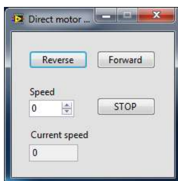
Figure 49. Direct motor control panel.
