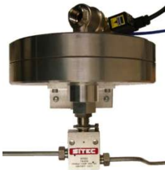
Figure 12. (Left) Photograph of a normally opened pneumatic diaphragm valve used as fast pressure jump valve. (Right) Schematic diagram of the fast opening pressure valve; (1) 6 bar air supply (controlled via solenoid valve); (2) quick air exhaust port; (3) pneumatic actuator diaphragm; (4) valve return spring; (5) high pressure ring seal; (6) high pressure valve pin; (7) high pressure valve seat; (8) high pressure inlet (high pressure should push valve pin out of seat); (9) high pressure outlet.
