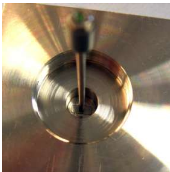
Figure 42. Photographs showing a Teflon sample being loaded into the pressure cell using the sample loading tool.
