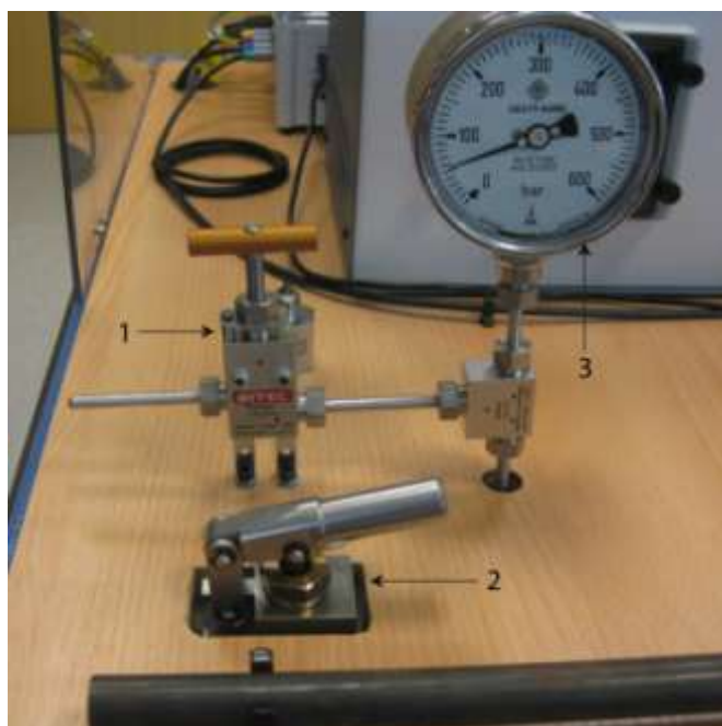
Figure 39. Location of (1) Medium pressure bleed valve V8, (2) 500 bar hand pump HP and (3) dial pressure gauge PG.
