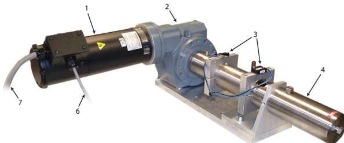
Figure 8. Photograph of high pressure generator (HPG); (1) Drive motor; (2) gear box; (3) limit switches; (4) high pressure generator barrel; (6) feedback tachometer cable; (7) motor power cable.
