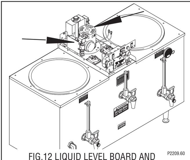
FIG.12 LIQUID LEVEL BOARD AND LEVEL PROBE
