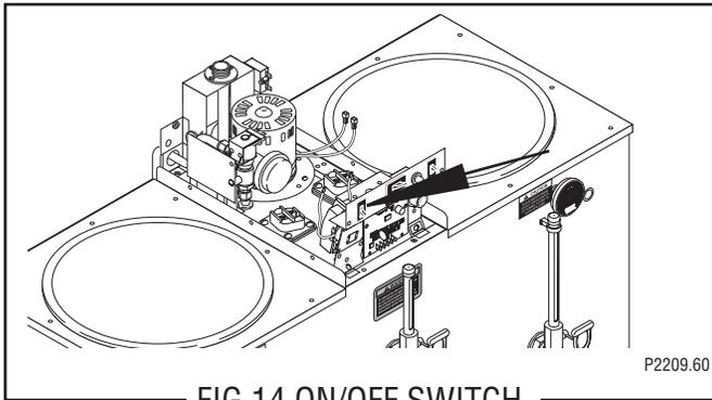
FIG.14 ON/OFF SWITCH
