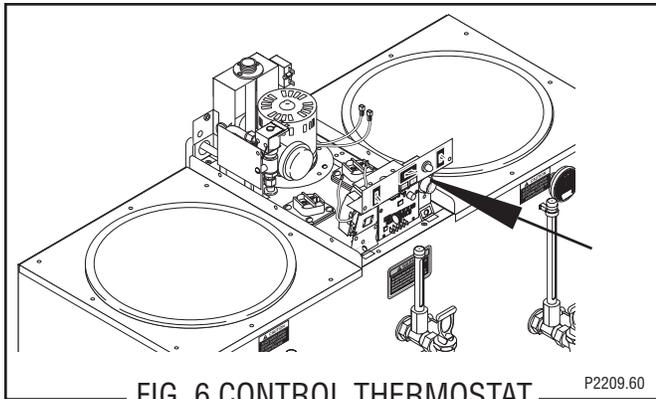
FIG. 6 CONTROL THERMOSTAT P2209.60
