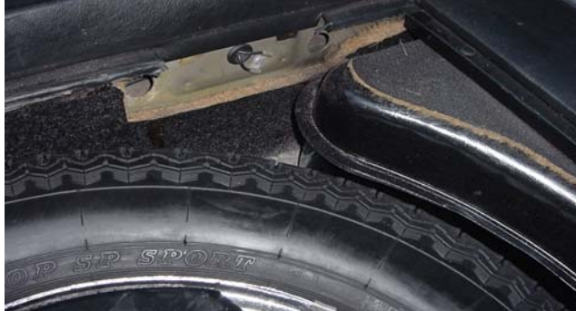
Sound deadening on rear vertical face of spare wheel well
