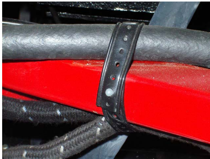
Wire Fixing Is Sometimes Used To Secure A/C Lines
