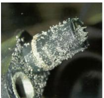
as wheel speed increases. Because the sensors are magnetic, they can attract metallic debris from semi-metallic brake linings and rotors that stick to the tip and interfere with the signal. If the ABS module doesn't see a clean WSS signal, it may think there's something wrong and set a wheel speed sensor code.
