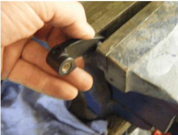
**Installation and removal of Mass Rivet(tip weight)**
