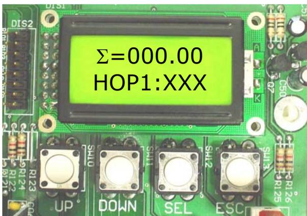
Use the UP and DOWN pushbuttons to increase or decrease the number shown until it is the desired quantity.
