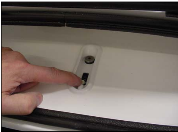
Power breaker in glove box
