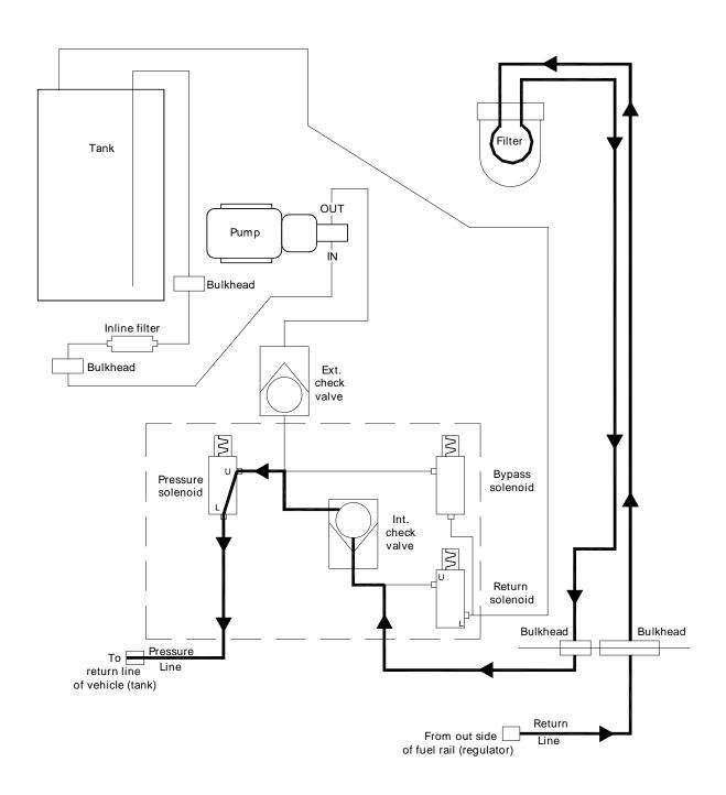
DIAGNOSTIC MODE ENGINE RUNNING NO KEYS "PRESSED"
