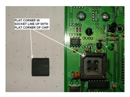
8. Insert new processor chip into socket.
