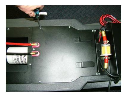
2. Remove the 4 nyloc nuts securing the front control board assembly using long extension with 3/8" Socket.
