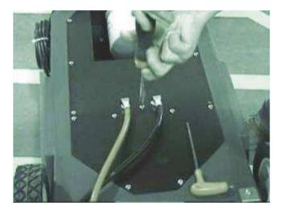
2. Remove the two (2) 5/32" Allen Head screws in filter cavity; a 4mm Allen Socket will also fit these 2 screw heads
