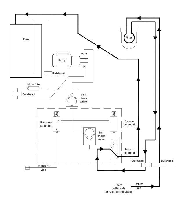
DIAGNOSTIC/FILL MODE ENGINE RUNNING FILL TANK "PRESSED"
