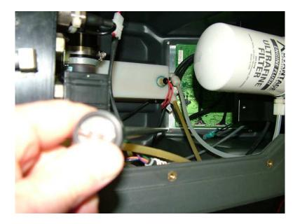
4. Disconnect wire connectors from board, if not marked J1, J2, J3 please mark before removal.
