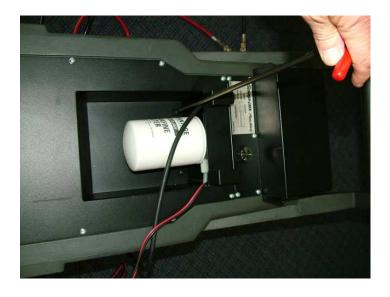
3. Remove the nickel plated hex head bolt threaded into the top of the black anodized Manifold Block (7/8" across the flats);
