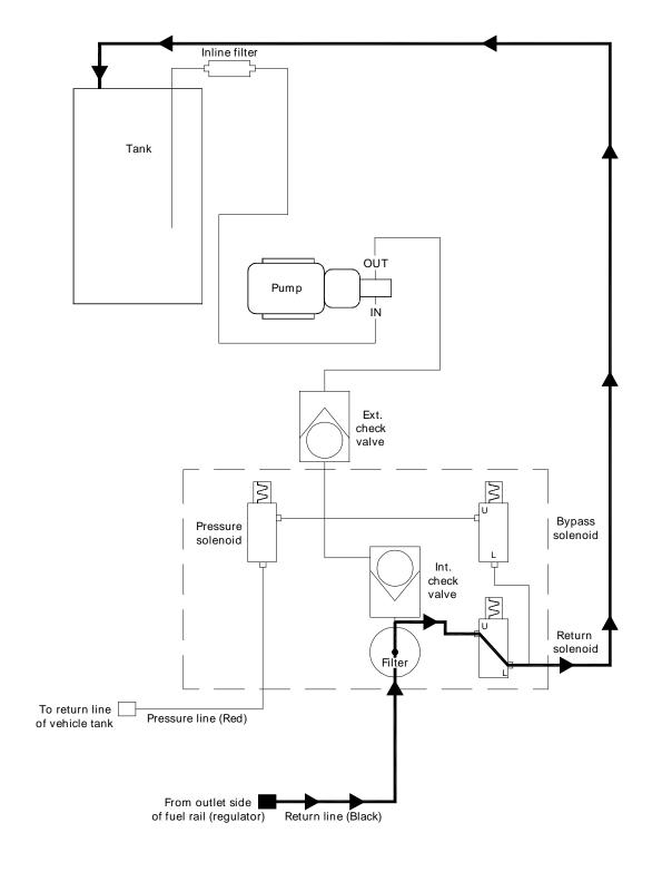
DIAGNOSTIC/FILL MODE ENGINE RUNNING FILL TANK "PRESSED"
