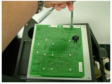
6. Remove processor chip from board using chip puller or tool that came with new chip.
