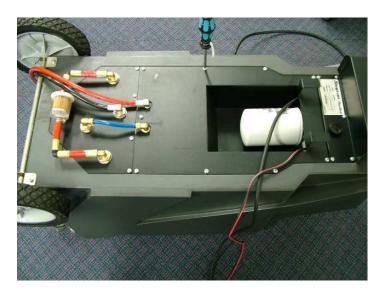
2. Remove the two (2) 5/32" Allen Head screws in filter cavity; a 4mm Allen Socket will also fit these 2 screw heads
