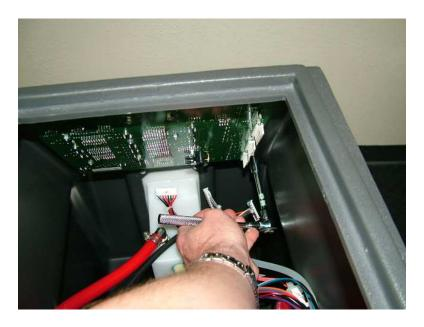
4. Place board assembly on top of unit and remove screws or nuts to separate circuit board from display panel.
