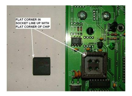
8. Insert new processor chip into socket.
