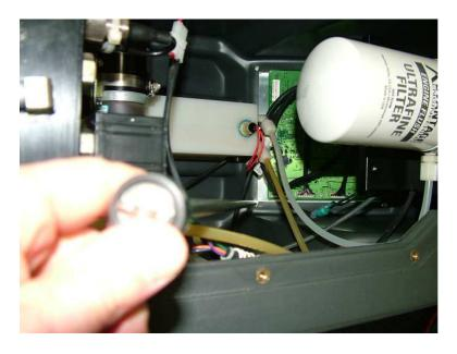
4. Disconnect wire connectors from board, if not marked J1, J2, J3 please mark before removal.
