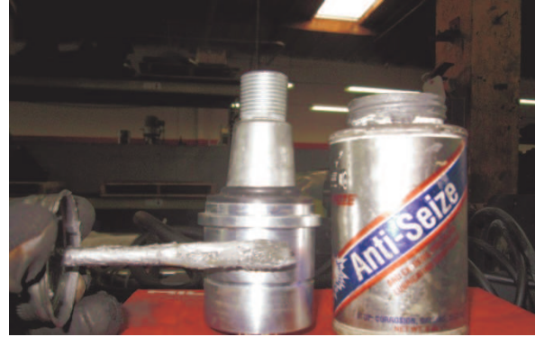
Figure 6, Placing Anti Seize on Ball Joints
