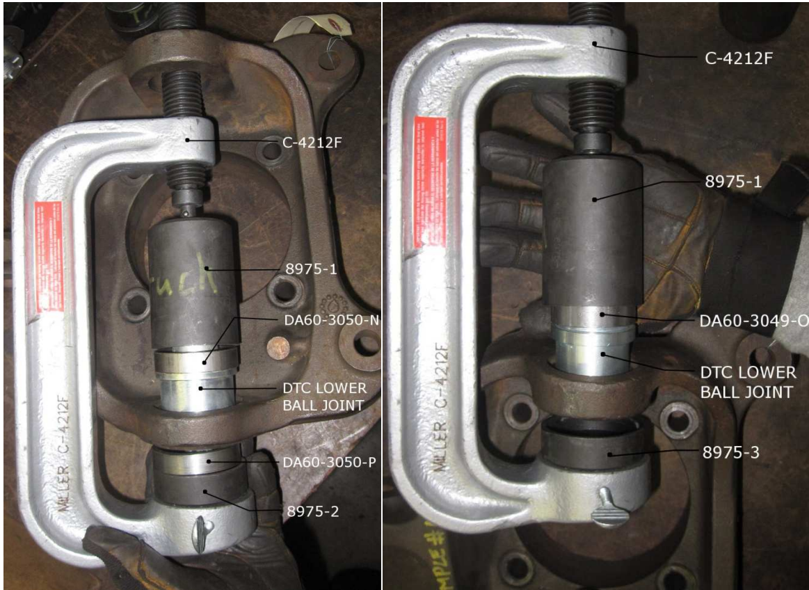
Figure 8, Pressing In Lower ProSteer Ball Joint
