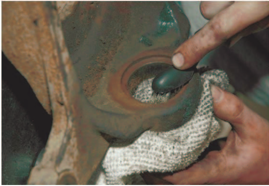
Figure 5, Cleaning the Knuckle
