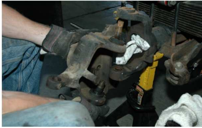
Figure 2, Removing the knuckle
