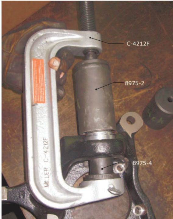
Figure 3, Removing the Upper Ball Joint
