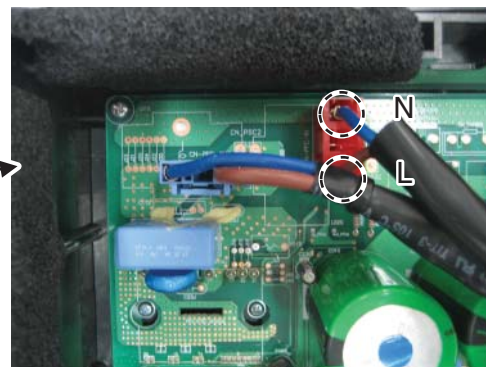
< Main PCB wiring Check Point >
