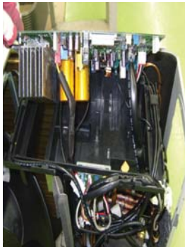
Raise PCB and take terminals from PCB
