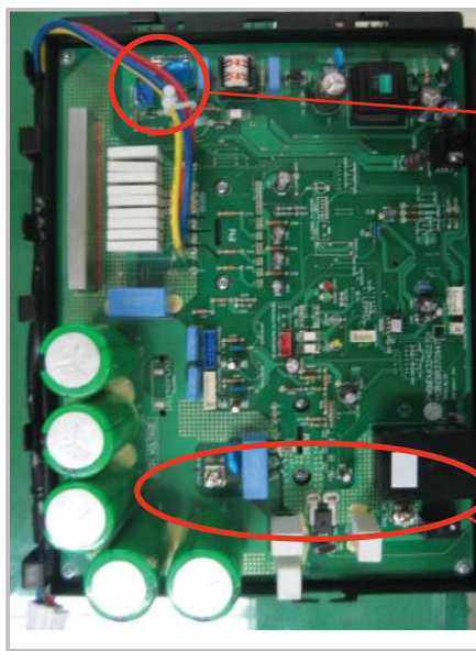
< Noise Filter wiring Check Point >
