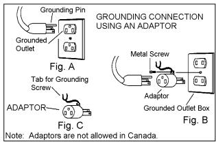
Improper connection of the equipmentgrounding conductor can result in a risk of electric shock. Check with a qualified electrician or service person if you are in doubt as to whether the outlet is properly grounded. Do not modify the plug provided with the appliance - if it will not fit the outlet, have a proper outlet installed by a qualified electrician.
