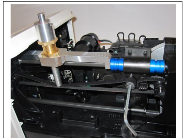
Use special tool to tighten the belt
