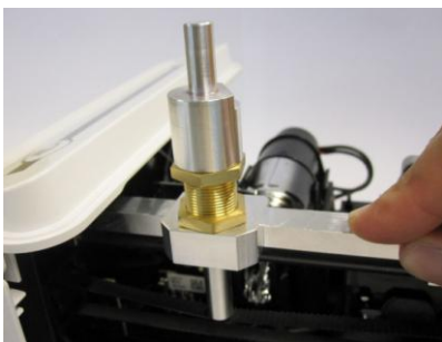
Push the tool against the shaft and belt.
