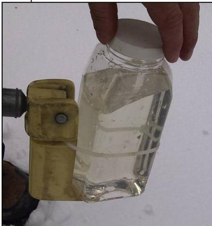
5. Make sure that the lid of the sample jar is not contaminated and that no dust or debris gets inside the sample. If something gets inside, a new sample bottle must be used and another sample taken
