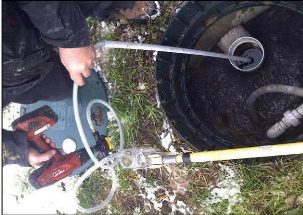
NOTE: The sampling pump and hose should be cleaned with a cleaning solution each morning prior to taking samples.
