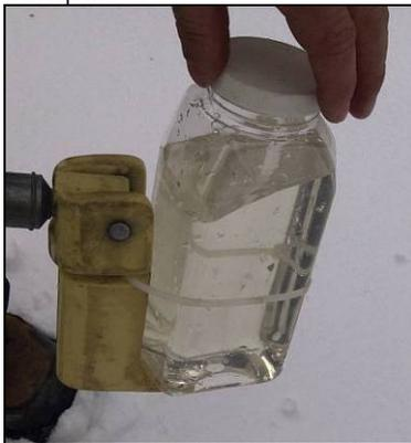
7. Make sure that the lid of the sample jar is not contaminated and that no dust or debris gets inside the sample. If something gets inside, a new sample bottle must be used and another sample taken
