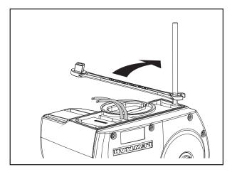
Next, using the wrench on the flats, tighten the studs until they bottom out in their holes. Do this to each of the studs in turn.
