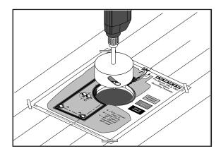
Using a 3/8" (10 mm) diameter drill, make the three holes for the mounting studs and two for the motor wires. With a 3" (76 mm) diameter hole saw, make the hole for the rode to pass through. When all the holes have been made, remove the template. To help avoid water absorption by the deck, apply an appropriate marine sealant to the freshly cut hole edges.
