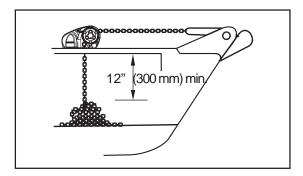
Place the windlass on the deck and decide upon a position for it with reference to the vessel's bow roller and the chain locker below. Rode lead from the roller should ideally be fed horizontally back to the top of the gypsy and along its centerline. There must be sufficient vertical fall for the chain or rope, even with a full locker, to draw the rode from the gypsy when hauling in.
