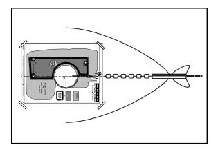
Place the mounting template on the deck or mounting pad in the desired position for the windlass and hold it in place using adhesive tape.
