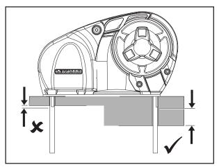
Place the base mat in position on the deck, optionally, apply a suitable sealant (DO NOT use a permanent adhesive/sealant, e.g., 5200) to the base of the windlass, any mounting pad and around the studs. **DO NOT get CAULK or SEALANT under the GEARTRAIN COVER (19)** as it makes it difficult to remove. Secure the windlass firmly to the deck from below, using the nuts and washers supplied.
