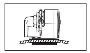
If the deck is not flat, a suitable mounting pad may be required to take up camber or sheer. Decks that are thin, or of foam or balsa laminate construction, will require reinforcement in order to spread the loads that will be applied to the deck while the windlass is in use. The standard 5/16" threaded mounting studs supplied suit deck and packing thickness of up to 3" (76 mm). These are adequate for most installations.
