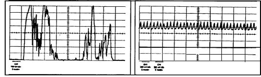
performance problem. Technician used a current probe and lab scope on fuel pump feed wire. See fuel pump waveform in picture to left.
