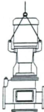
Figure 2-1. Typical lifting method using lifting brackets.
