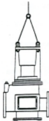
Figure 2-2. Typical lifting method using eye bolts.
