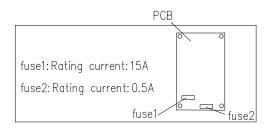
According the figure, take out the fuse1, replace a new one
