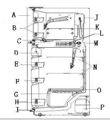
A=freezer door B=bottle shelf C=cold air suction hole D=egg box cover E=bottle shelf F=bottle shelf G=vegetable container H=bottle shelf I=Ref door J=FRZ fan motor K=wire L= evaporator N=Ref air passage O=vegetable container cover P= compressor
