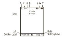
1 Signal Strength Indicator: Vertical bars show the strength of the network connection. You can't make or receive calls when shows.
