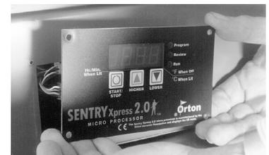
**3** Look at the back of the controller. You will find a set of connector pins near the bottom labeled “C/F.” When a jumper is placed on the C/F pins, the display reads °F. When the jumper is removed, display reads °C. Remove or insert the jumper as desired. (You can purchase the jumper from a computer supply store if necessary.)
