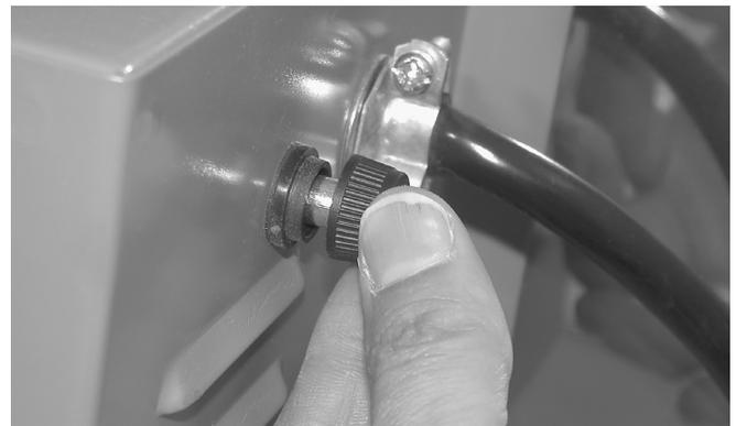
■ What size fuse are you using? Correct fuse: AGC ½ A 250V AC
