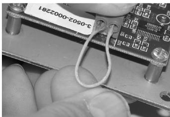
1 UNPLUG the kiln or disconnect the power. Remove the controller. Remove the two thermocouple wires from the back of the controller.
