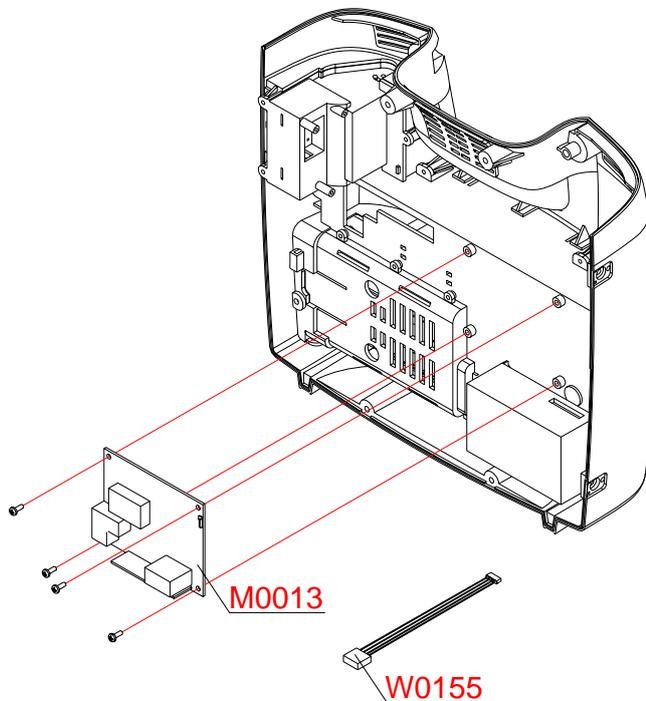
**Figure 23. Rear case disassembly – EtCO<sub>2</sub> module**
