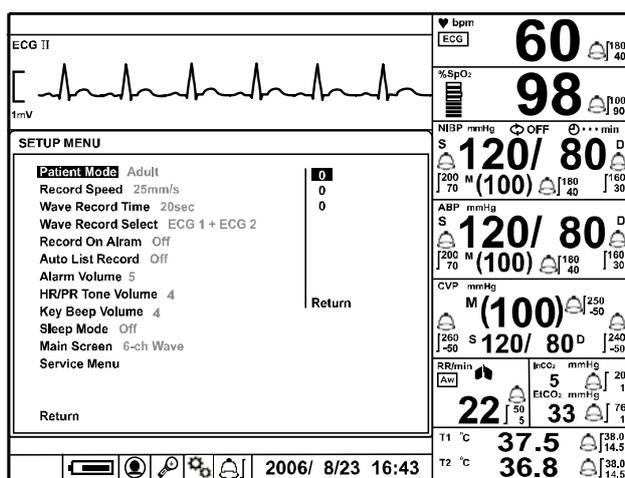
Figure 11. The access of Service Menu via Set-up menu
