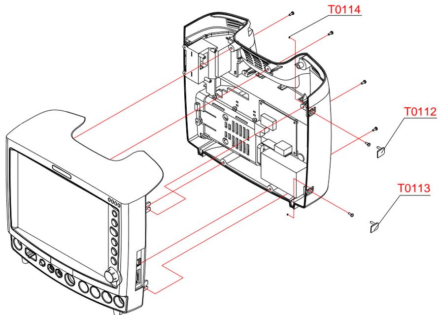
**Figure 17. Monitor Disassembly**
