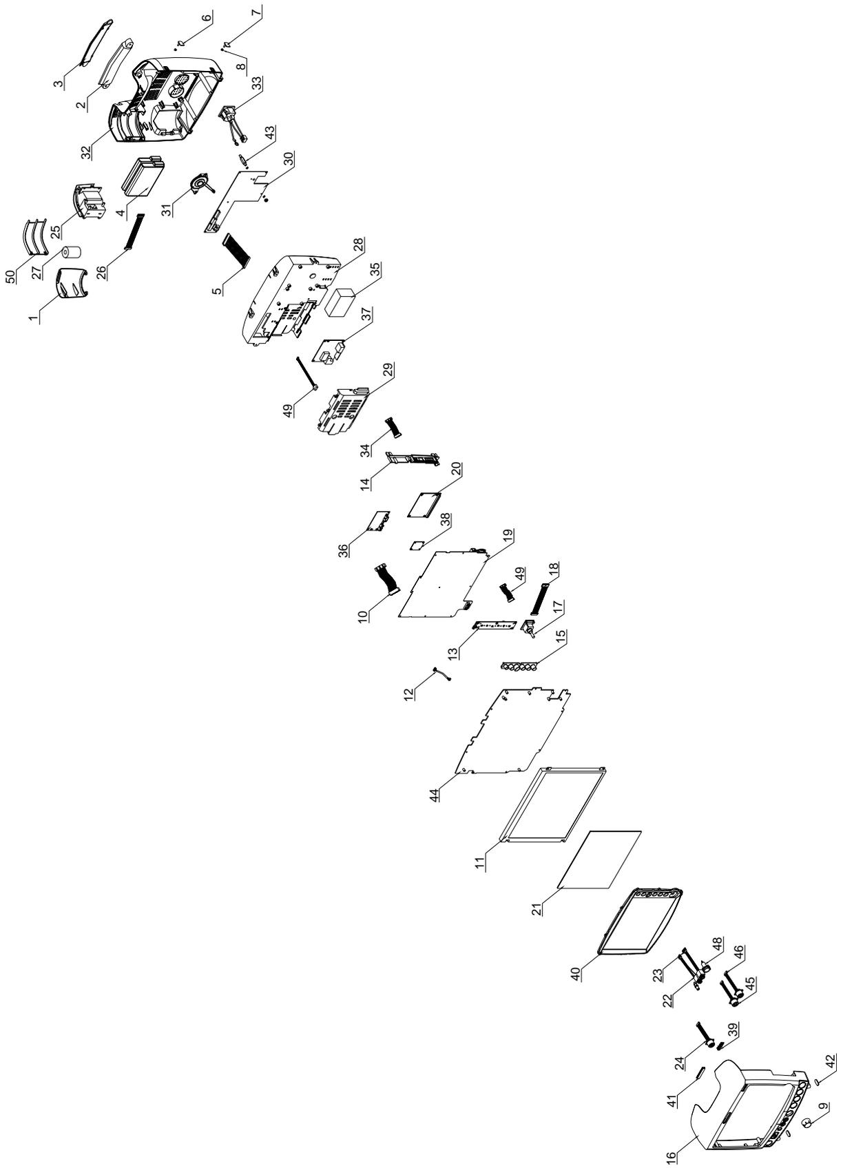
Figure 27. YM6000 Exploded View – Spare Parts
