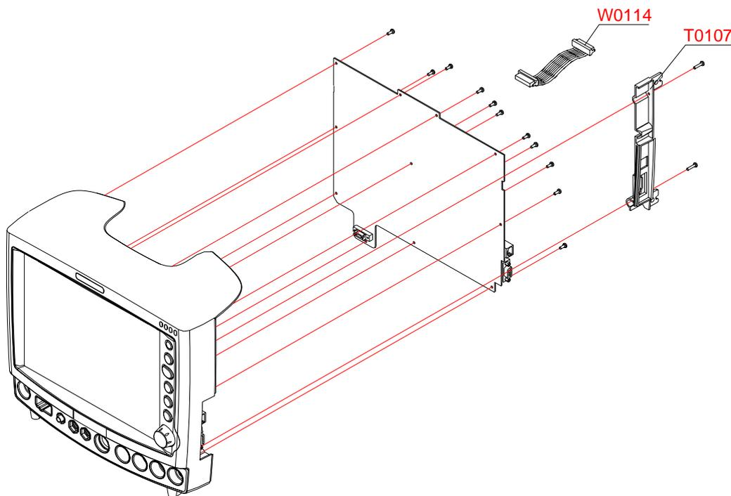
Figure 18. Front Case Disassembly – Side connector holder and Main board
