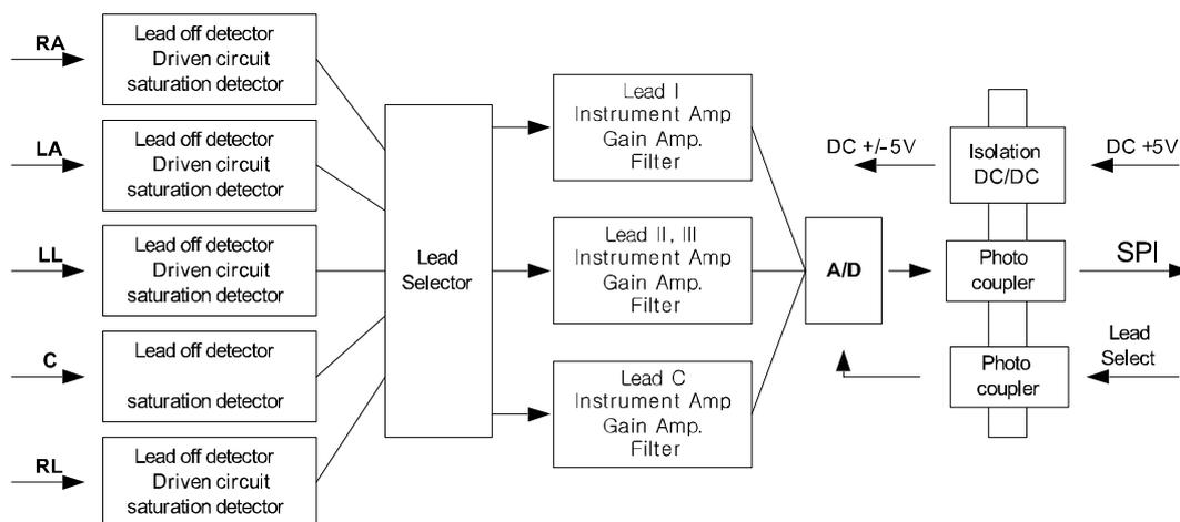
Figure 38. ECG Unit Block Diagram
