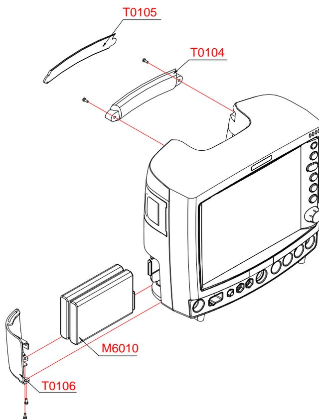
Figure 16. Battery and Handle Disassembly
