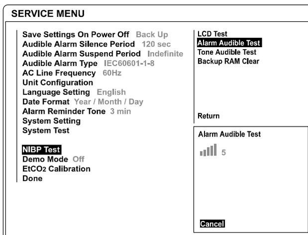
Figure 5. Alarm Audible Test
