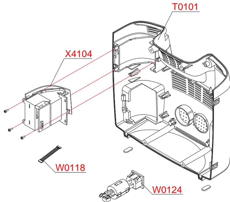
Figure 26. Rear case disassembly – Printer module and AC inlet
