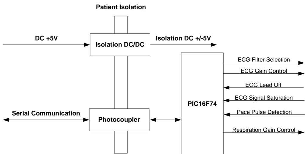
Figure 43. Analog Control Unit Block Diagram
