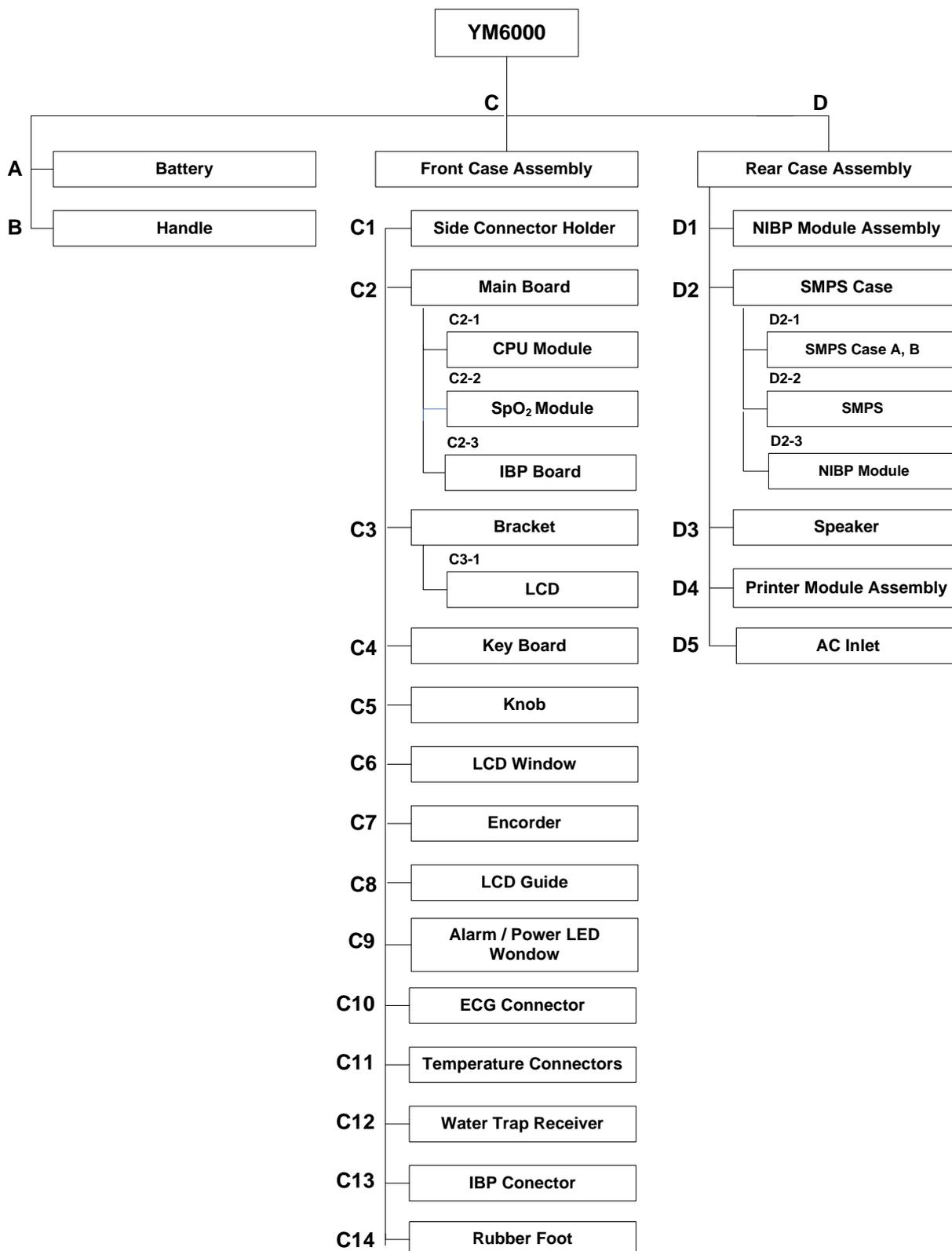
Figure 15. Disassembly Sequence Flow Chart
