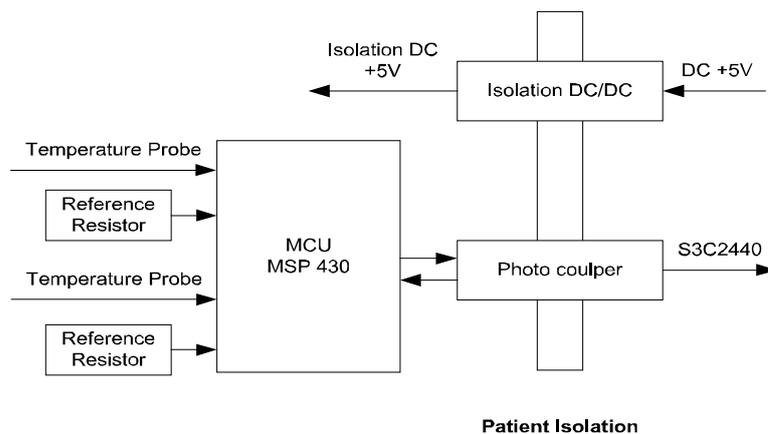
Figure 41. Temperature Unit Block Diagram
