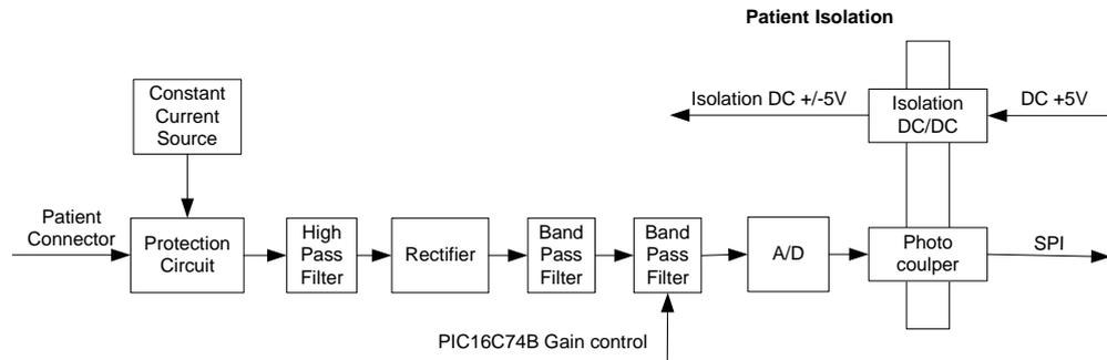
Figure 39. Respiration Unit Block Diagram
