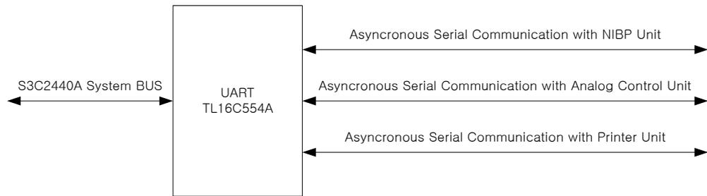
Figure 33. Communication Unit Block Diagram
