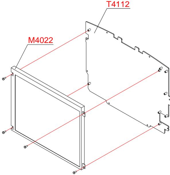
Figure 21. Front Case Disassembly – sLCD and Bracket
