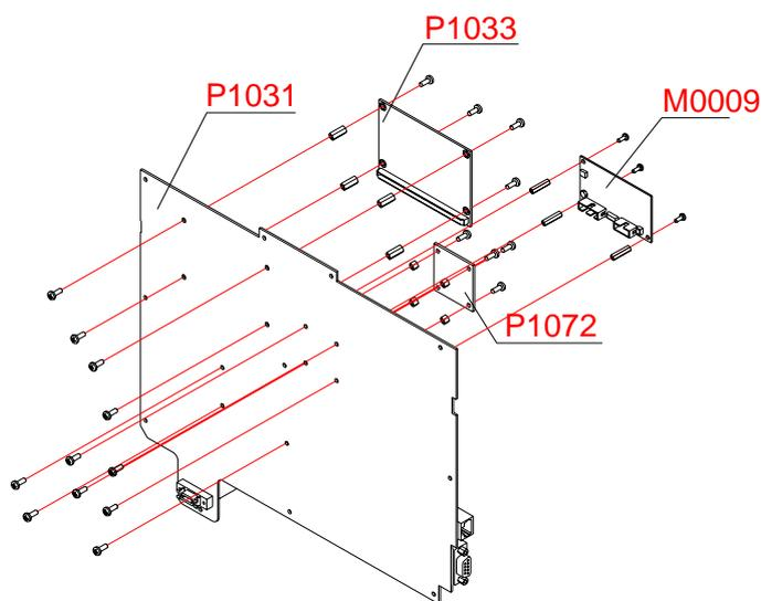
Figure 19. Front case disassembly – CPU module, SpO<sub>2</sub> module and IBP board
