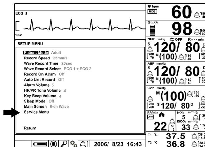
Figure 10. The access of Service Menu via Set-up menu
