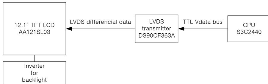
Figure 34. GUI Unit Block Diagram
