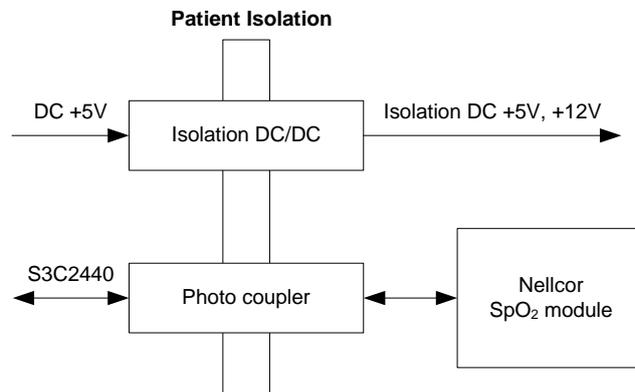
Figure 40. SpO<sub>2</sub> Unit Block Diagram
