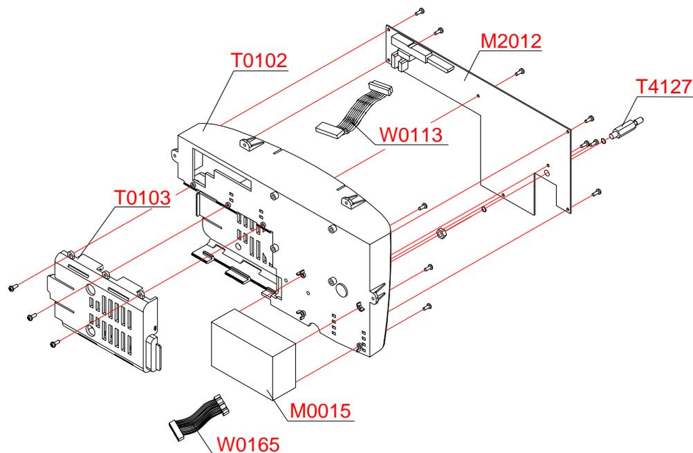
**Figure 25. Rear case disassembly –SMPS case, SMPS and NIBP module**
