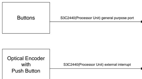
Figure 31. User-Control Unit Block Diagram
