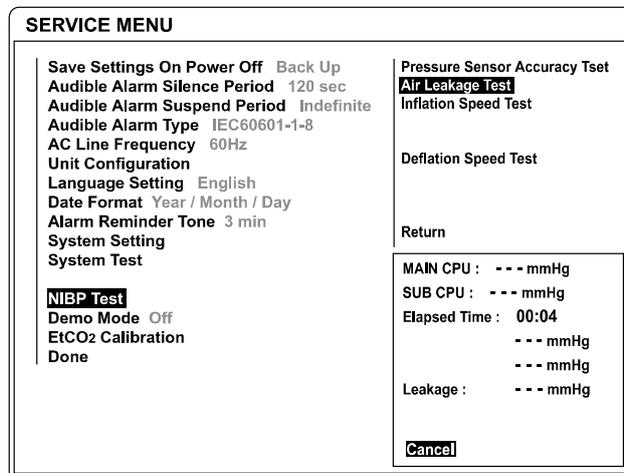
Figure 9. Air Leakage Test
