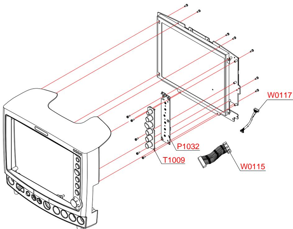
Figure 20. Front Case Disassembly –Bracket and Key board
