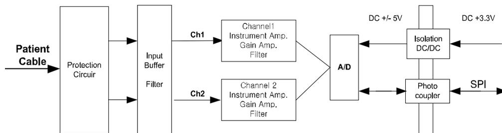
Figure 42. IBP Unit Block Diagram
