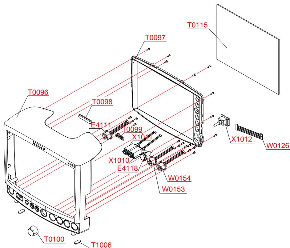
Figure 22. Front Case Disassembly – Knob, LCD window, Encoder assembly and Connectors
