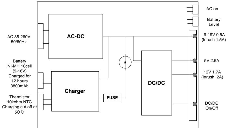
Figure 29. Power Unit Block Diagram
