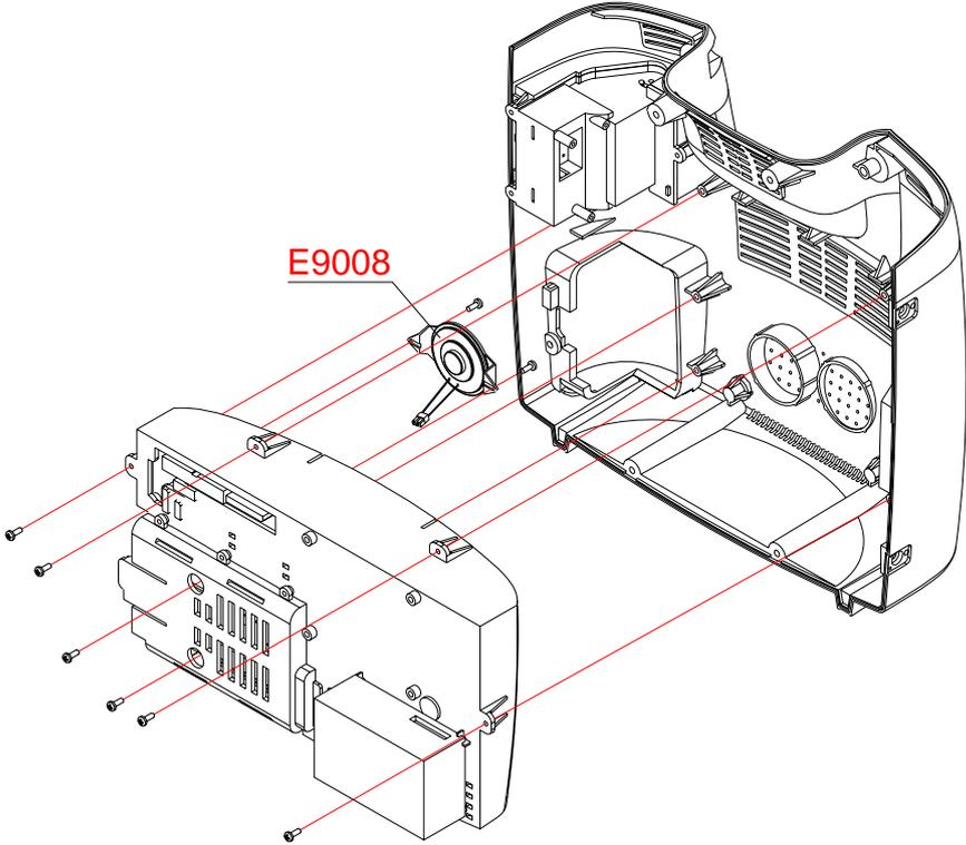
Figure 24. Rear case disassembly – Speaker
