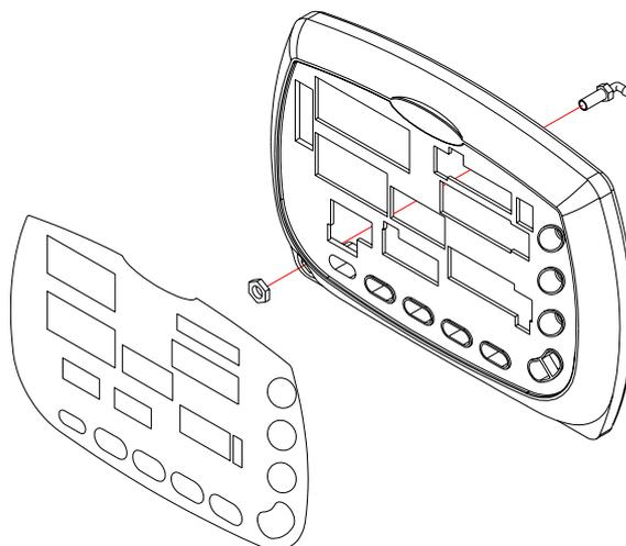
**Figure 24. Front Case Disassembly – Overlay, NIBP cuff hose connector**
