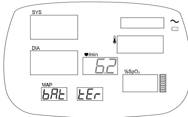
Figure 6. Battery Voltage Level
