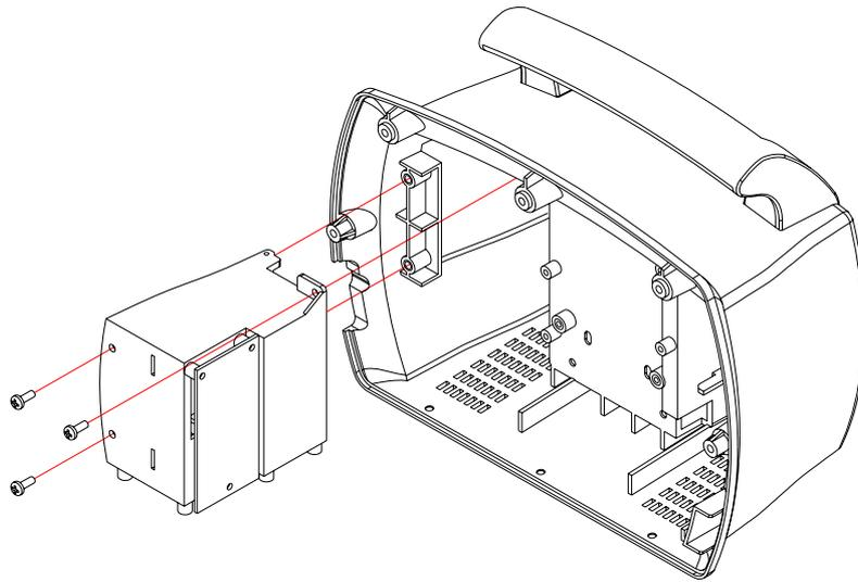
Figure 27. Rear Case Disassembly- Printer
