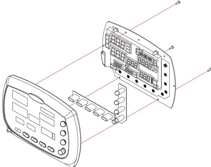
**Figure 22. Front Case Disassembly**
