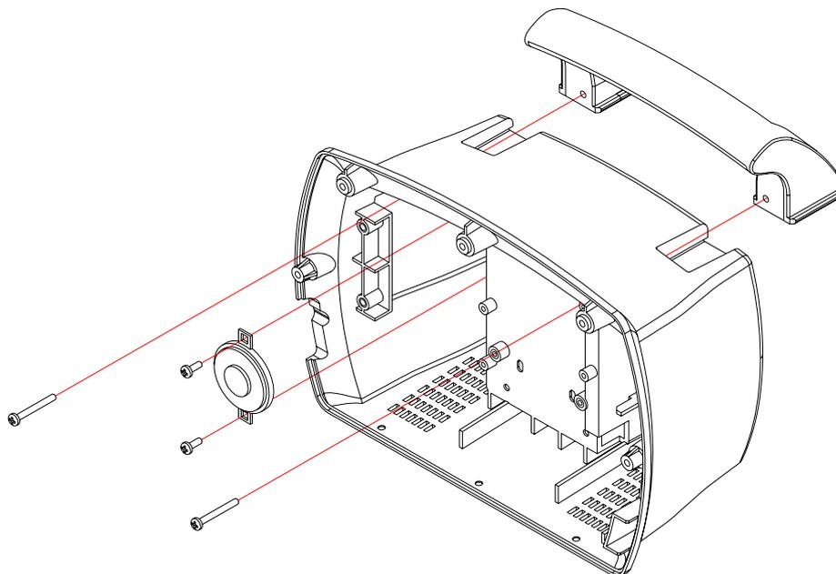
Figure 28. Rear Case Disassembly – Speaker, Handle, etc
