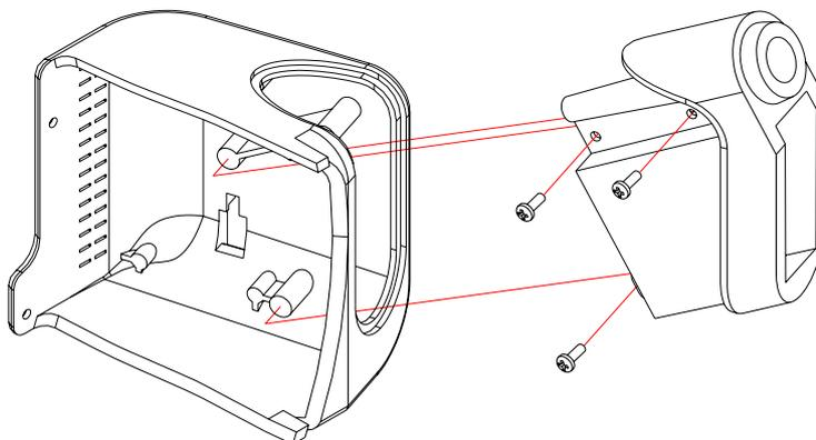
**Figure 30. Temperature Case Disassembly**
