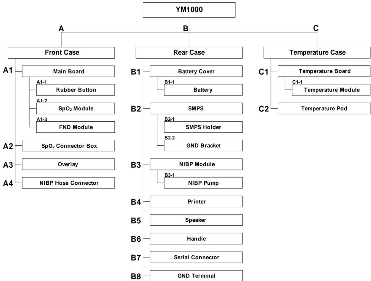
Figure 19. Disassembly Sequence Flow Chart
