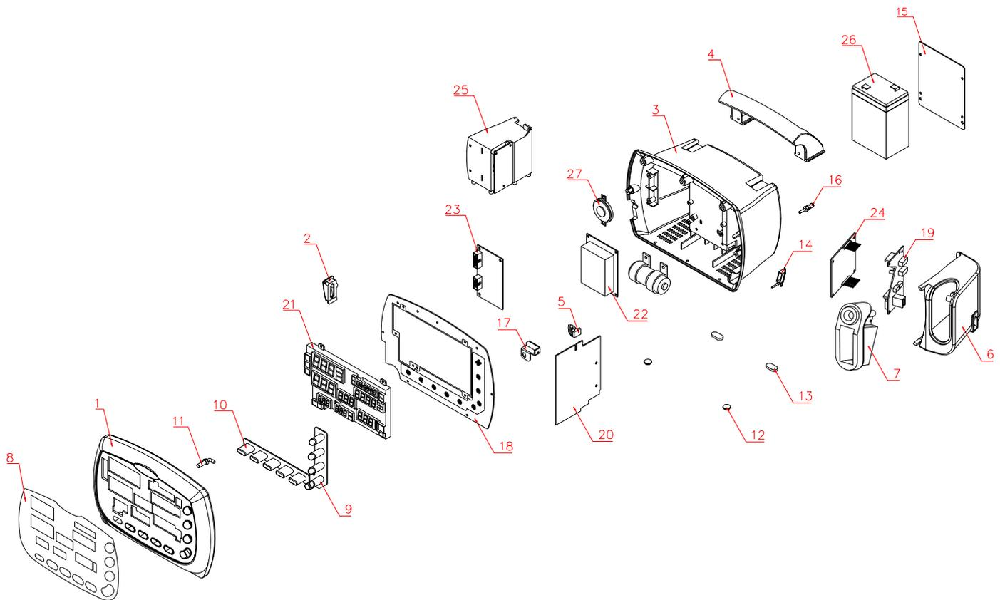
Figure 32. YM1000 Exploded View – Spare Parts
