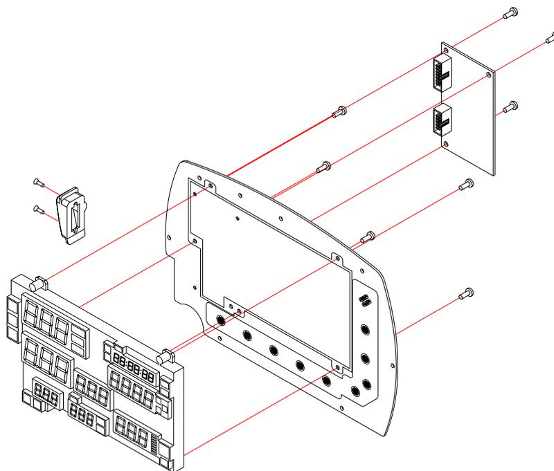
Figure 23. Main BD, SpO<sub>2</sub>, FND modules Disassembly
