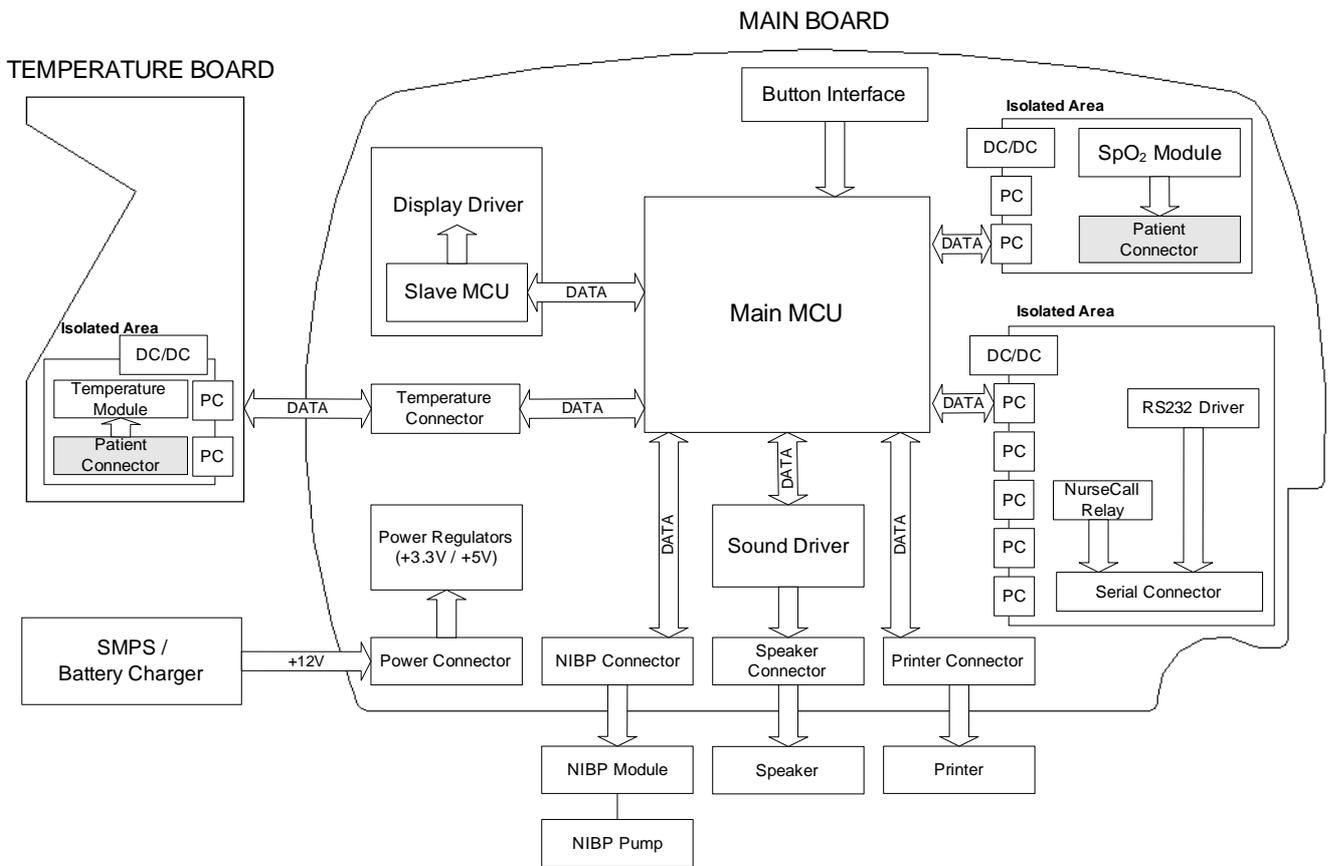
Figure 33. YM1000 System Block Diagram
