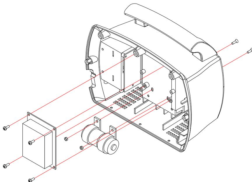
**Figure 26. Rear Case Disassembly- NIBP module**
