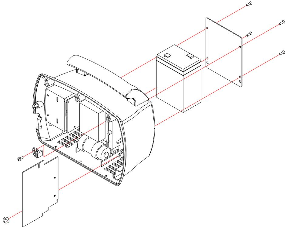
Figure 25. Rear Case Disassembly- Battery, SMPS
