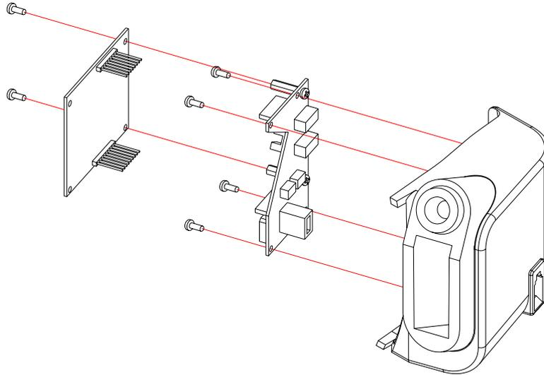
**Figure 29. Temperature Case Disassembly – Temperature Module**
