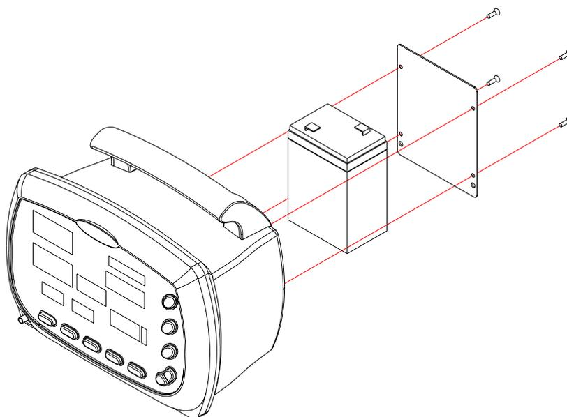
Figure 20. Battery Disassembly
