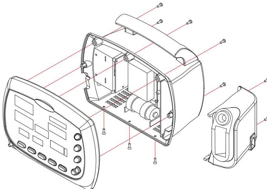
Figure 21. Monitor Disassembly
